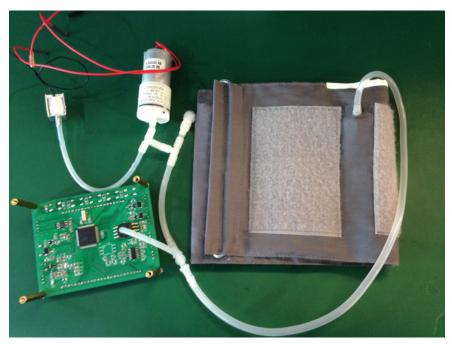
Figure 6. Connection of Cuff, Pump, Valve, and Sensor for Gas Path
