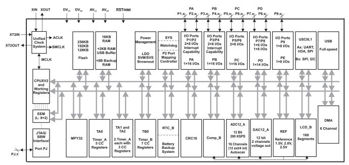
Figure 2. Functional Block Diagram for MSP430F6638
