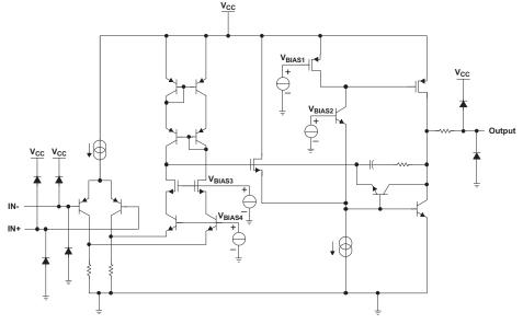
Figure 3. LMV324 Detailed Schematic
