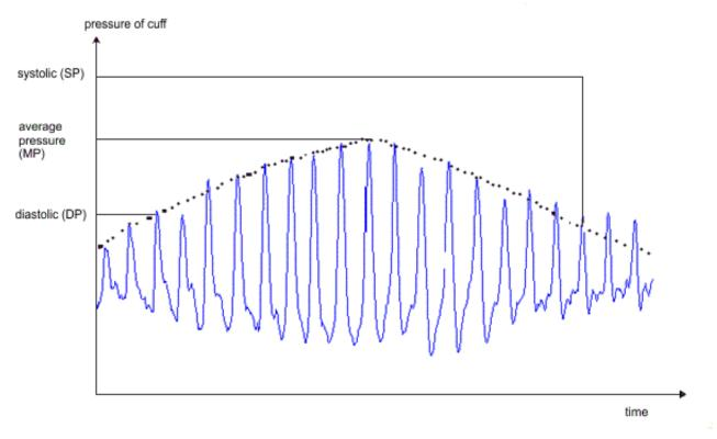
Figure 5. Oscillation Method to Get Blood Pressure
