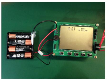
Figure 8. Connect to the Board
