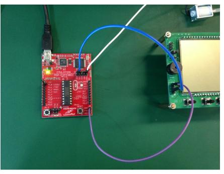
Figure 9. Raw Data Readout Through UART
