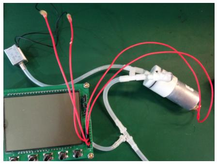
Figure 7. Pump and Valve Electronic Connection to the Board
