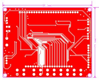
Figure 16. Top Silkscreen layer of PCB
