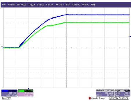
3.4 Start Up @  $528V_{AC}$  ( $528V_{AC}$  is generated by an  $264V_{AC}$  with a voltage doubler circuit): no load.
