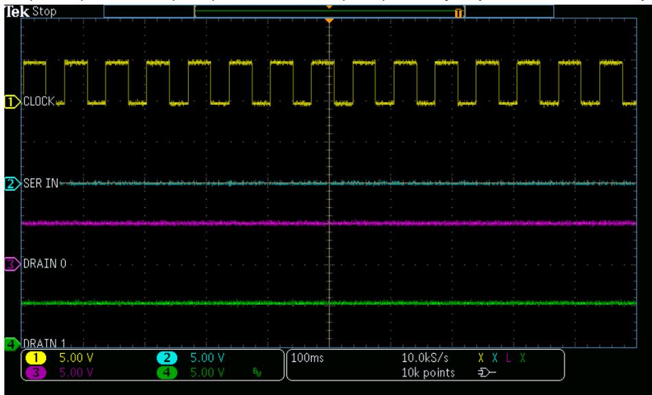
**D. Oscilloscope captures of ROLLING operation**
