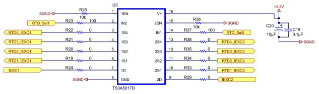
Figure 16. Multiplexer Section
