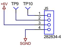
Figure 21. DC Input Connector
