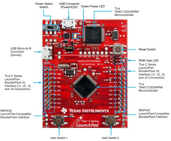
Figure 22. Tiva C Series TM4C123G LaunchPad Evaluation Board
