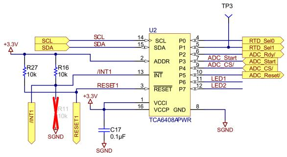
Figure 18. I2C I/O Expander
