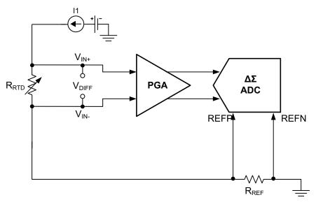
Figure 2. Simplified Circuit for RTD Ratiometric Measurement
