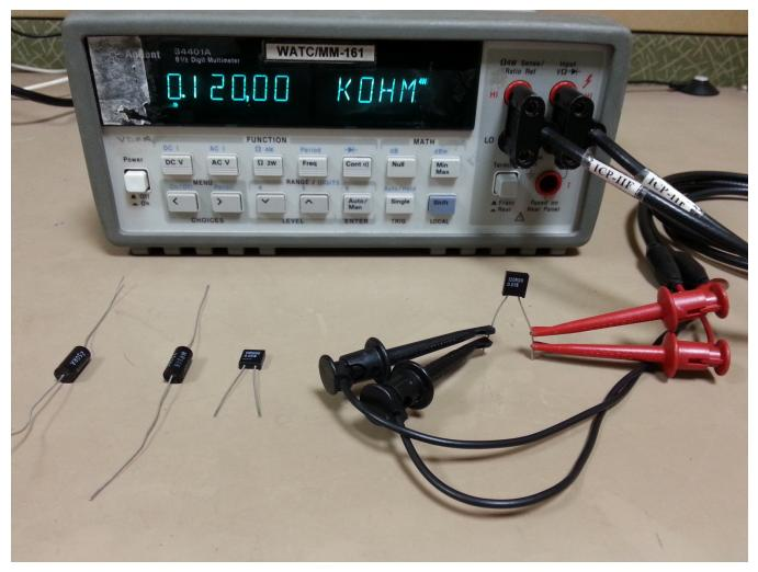
Figure 25. 4-Wire Resistance Measurement Using 61/2-Digit Multimeter
