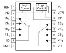
Figure 15. Pin Configuration View of TS3A5017D
