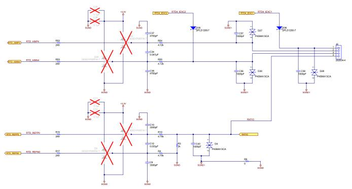
Figure 12. Common-Mode and Differential-Mode Filters Implemented in Design for RTD
