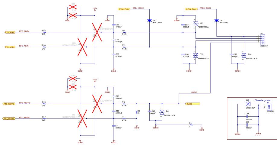
Figure 28. RTD4 and Ratiometric Measurement
