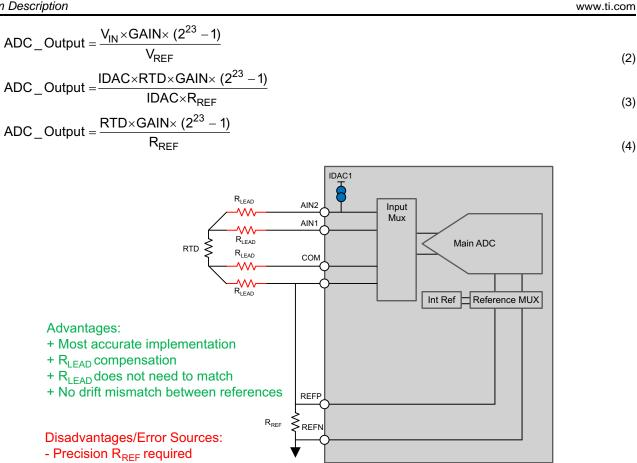
Figure 3. Ratiometric 4-Wire Operation
