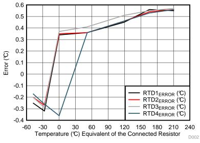
Figure 26. RTD Measurement Accuracy
