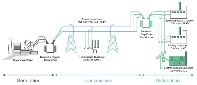
Figure 5. Smart Grid — Generation to Distribution
