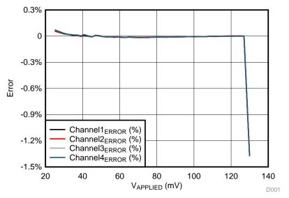
Figure 24. ADC Linearity Performance After Applying Gain Factor
