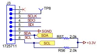
Figure 14. J3 Connector for SPI and I2C Interface With External Devices
