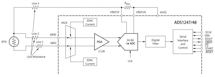
Figure 9. 3-Wire RTD Measurement Circuit Diagram
