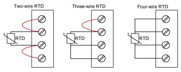
Figure 4. Different RTD Input Connections
