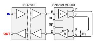
Figure 3: Multipoint eye diagram measurement
