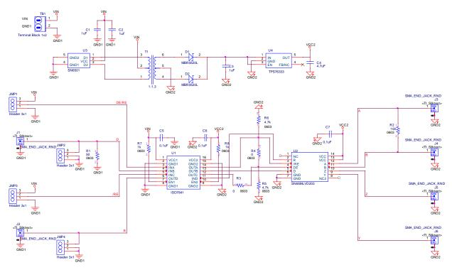
Figure 10: Reinforced isolated MLVDS transceiver
