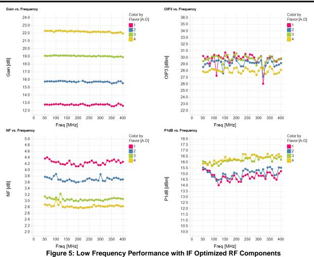
This configuration provides good RF performance from 50 MHz to 400 MHz.
