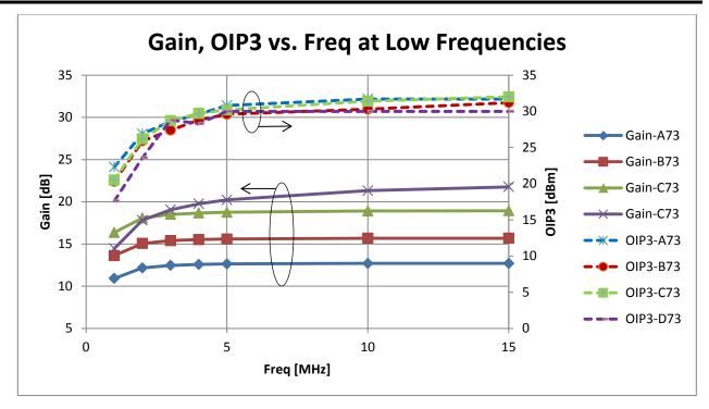
Figure 4: Gain and OIP3 Response down to 1 MHz
