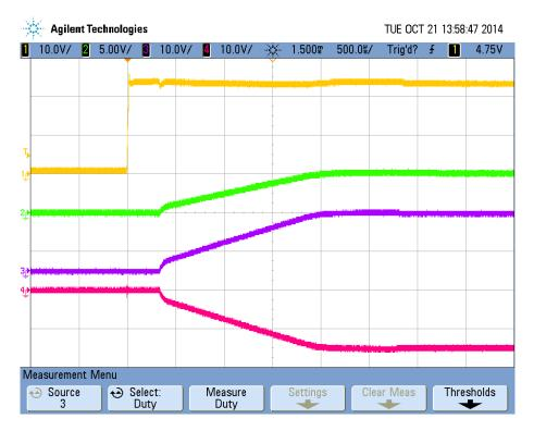
Figure 9 Start up into full load at 24Vin
