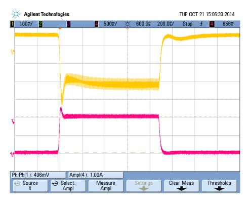
Figure 15 5V output load transient
