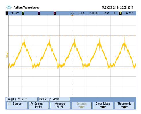
Figure 18 5V output ripple at full load, 24Vin
