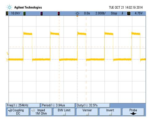
Figure 11 Switching waveform at full load, 24Vin
