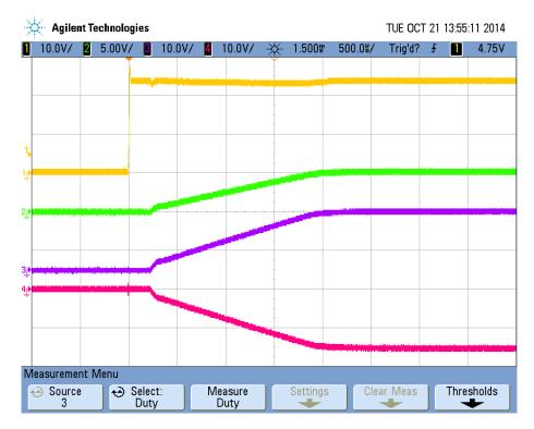
Figure 8 Start up into no load at 24Vin
