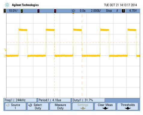
Figure 10 Switching waveform at no load, 24Vin
