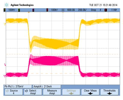
Figure 16 +15V output load transient
