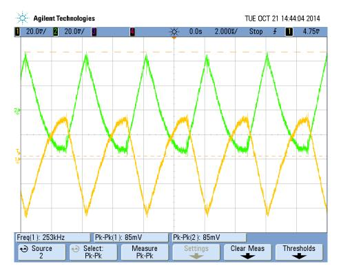
Figure 19 +/-15V output ripples at full load, 24Vin
