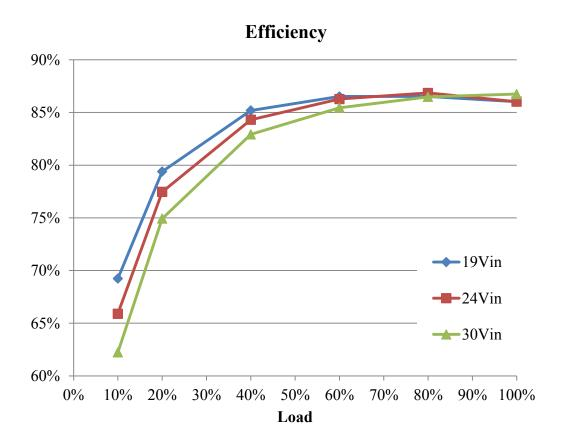
Figure 3 Total efficiency under balanced load
