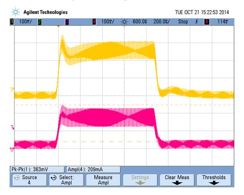
Figure 17 -15V output load transient
