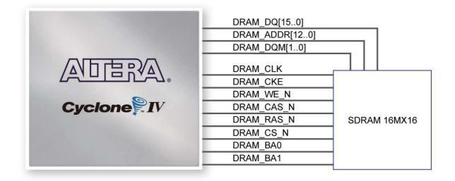
Figure 3-6 Connections between FPGA and SDRAM
