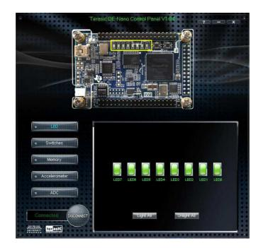
Figure 4-1 The DE0-Nano Control Panel
