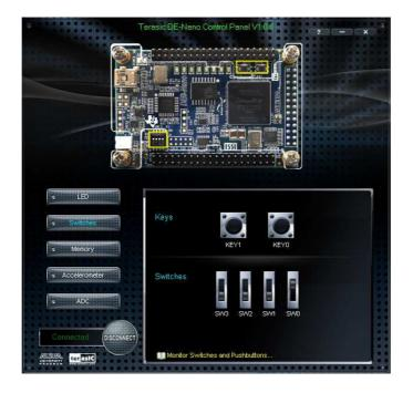
Figure 4-4 Monitoring switches and buttons
