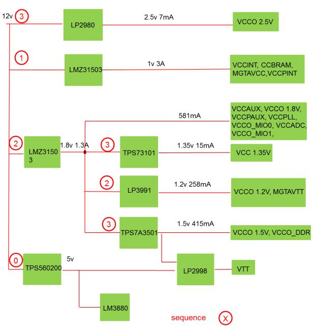
Figure 1. Block Diagram
