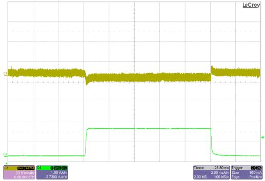
Figure 12. VIN = 12V, VCCINT Load Transient slew rate=1A/us
