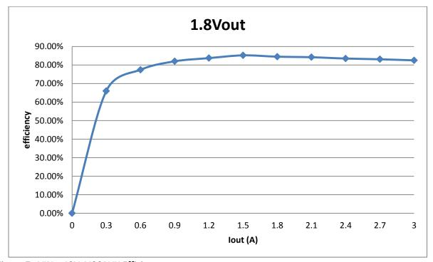
Figure 7. VIN = 12V, VCCAUX Efficiency
