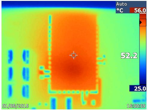
Figure 15. VIN = 12V, VCCAUX Thermal Image @ Full Load
