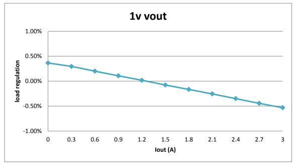
Figure 8. VIN = 12V, VCCINT Load Regulation
