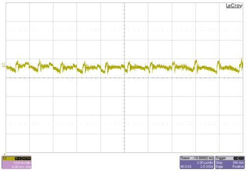
Figure 10. VIN = 12V, VCCINT Output Ripple @ IOUT = 3A
