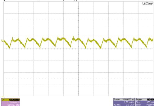
Figure 11. VIN = 12V, VCCAUX Output Ripple @ IOUT = 3A
