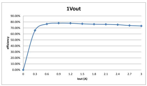
Figure 6. VIN = 12V, VCCINT Efficiency
