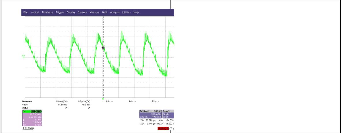
3.3V 220Vac 110mA Load Ripple and Noise
