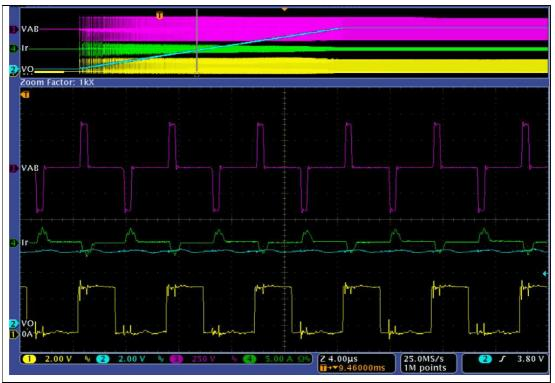
Phase shift mode in low output voltage. Vin=380Vdc, Vo=12V, Io=10A
