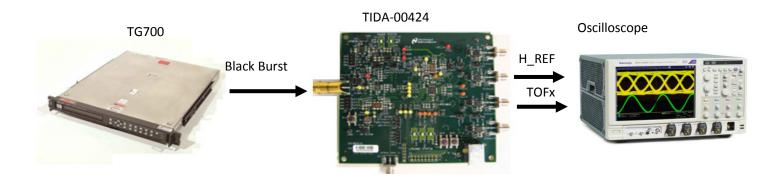
Figure 1. Test setup
