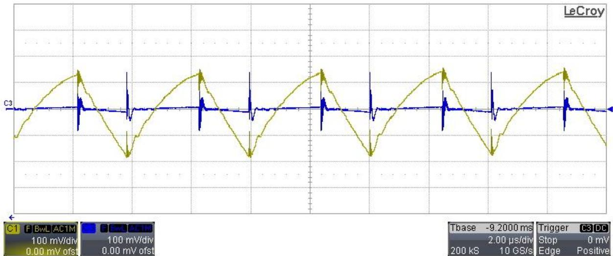
**Ch.3: Ripple voltage on C100 (100mV/div, 2us/div, 20MHz BWL, AC coupling)**
