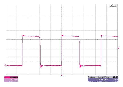
The photo below shows the FET switching voltage. The input voltage is 3.6V and the output is loaded to 0.43A. The converter is operating in DCM. (2V/DIV, 1uS/DIV)
