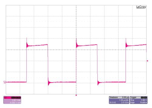
The photo below shows the FET switching voltage. The input voltage is 3.6V and the output is loaded to 3.25A. (2V/DIV, 1uS/DIV)
