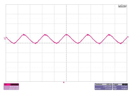
The 3.3V output ripple voltage (AC coupled) is shown in the figure below. The image was taken with the output loaded to 3.25A. The input voltage is set to 3.3V. (50mV/DIV, 2uS/DIV)
