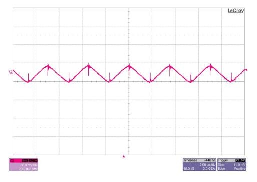
The 3.3V output ripple voltage (AC coupled) is shown in the figure below. The image was taken with the output loaded to 1A. The input voltage is set to 3.3V. (50mV/DIV, 2uS/DIV)
