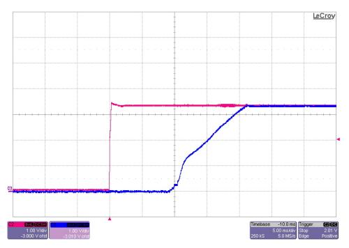
The photo below shows the output voltage startup waveform after the application of 3.3V in. The 3.3V output was loaded to 3.25A. (1V/DIV, 5mS/DIV)
