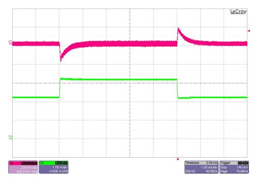
The photo below shows the output voltage (ac coupled) when the load current is stepped between 1.5A and 3A. Vin = 3.3V. (200mV/DIV, 1A/DIV, 1mS/DIV)
