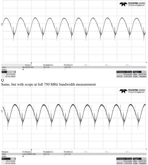
Ripple out at 1.5A load measured at main output J2 terminals: Vin is 32V Vout is 4.985V 106mV p-p ripple, slightly less at lower Vin's
