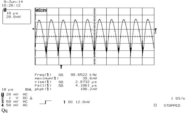
Same 32Vin, but load cut in half to 0.75A off: Ripple here 58mV p-p
