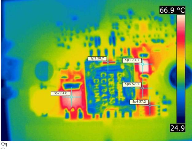
PMP11012: 32Vin Flyback to 5V 2.5A 100kHz no fan:Clamp resistor R1 hottest at 69 degrees C Sp1; main output diode D1 at 63 degrees C Sp2; ,xformer winding 56 Sp3; main Q1 switch 51 Sp4; output cap area 57 Sp5; ambient 21 deg. C
