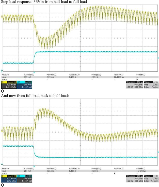
Step load response: 36Vin from half load to full load
