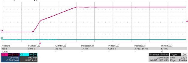
Start up: 36Vin applied with no load: Overshoot is 17mV max
