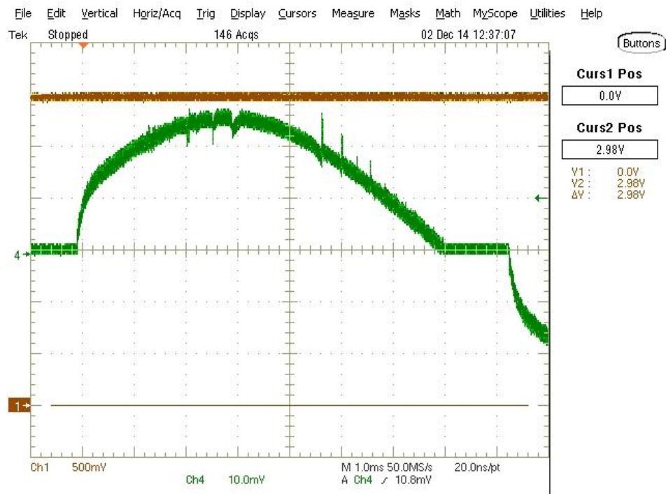
Figure 12: TPS92410 Vref, external 3.0 volt reference used for TSN, ADIM
