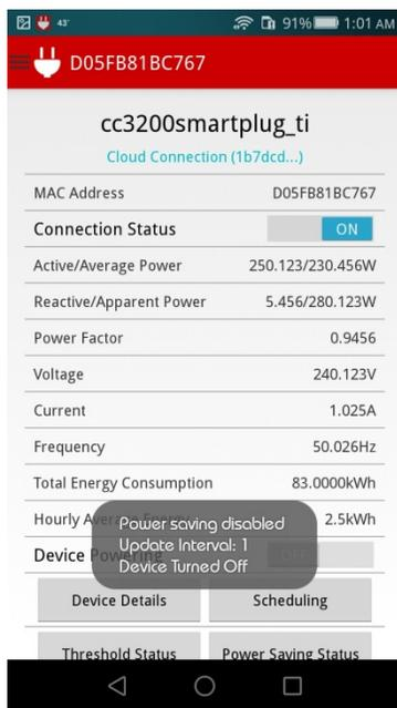
Figure 11. Device Screen With Cloud Connection Running
