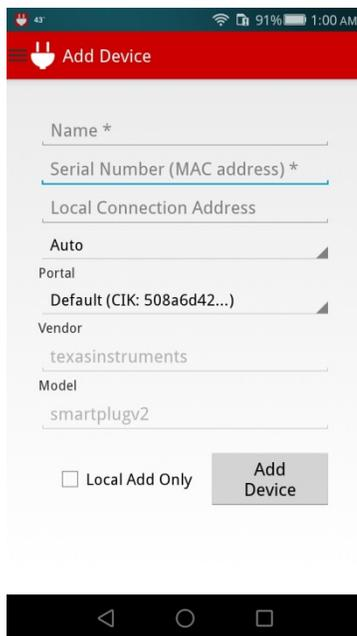
**Figure 9. Adding a Device Manually by Entering Information**
