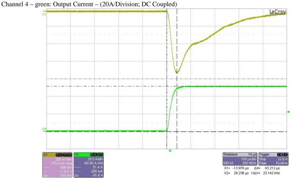
13.5Vout transient response showing 0A-50A load step
