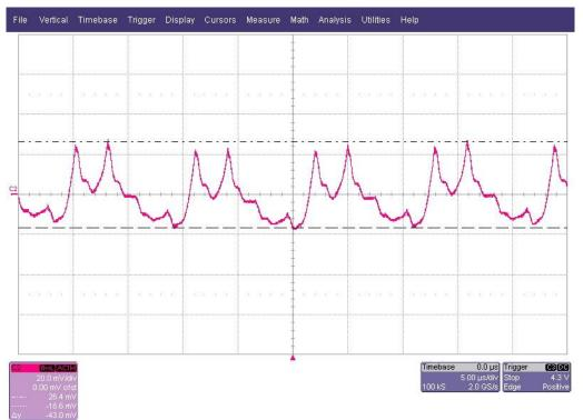
13.5Vout Voltage ripple at 0A load (Vrip=43mv pk-pk) Channel 1 – Yellow: Output Voltage – (50mv/Division; AC Coupled) (5us/div)
