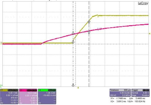
13.5V Output showing rise time from 0V-11V is less than 20msec
