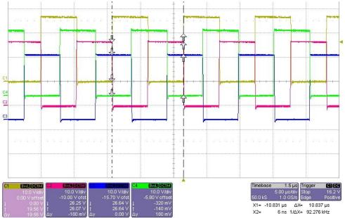
4Phase operation; 90 deg phase shift at 50% DC;  $F_{sw} = \sim 100 KHz$
