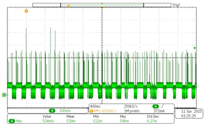
Figure 23. 3.3-V Supply Current Peaks During Wi-Fi Transmission
