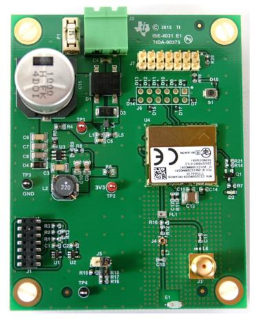
Figure 1. UART to Wi-Fi Bridge With 24-V AC Power
