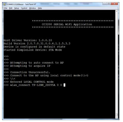
Figure 17. Setting Up the Access Point SSID
