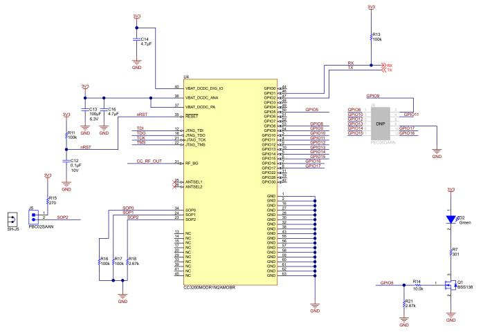
Figure 10. CC3200MOD Schematic
