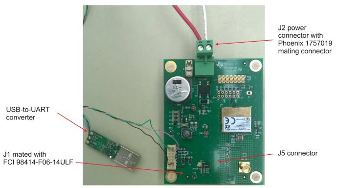
Figure 14. Board With Power and FCI Connector Plus USB-to-UART Converter
