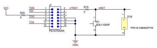
Figure 11. JTAG Connector Schematic
