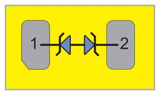
Figure 7. TPD1E10B06 Device Configuration
