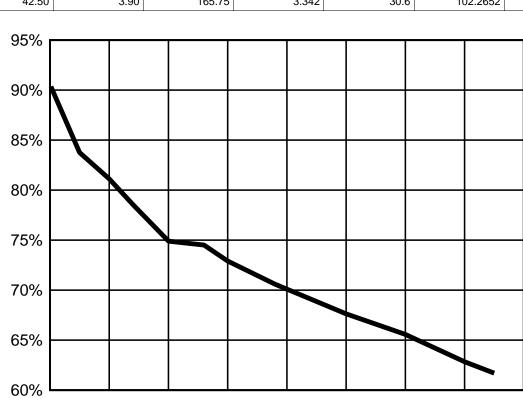
Figure 21. Power Supply Efficiency for UART Idle
