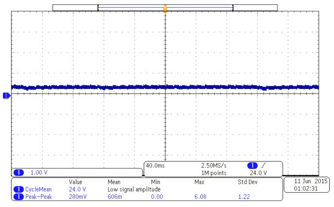
Figure 25. Ripple Voltage at C15 for an 18-V AC, 50-Hz Input
