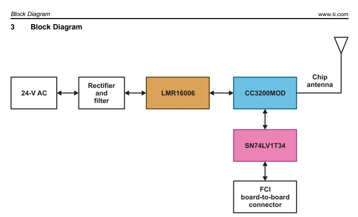
Figure 2. TIDA-00375 Block Diagram
