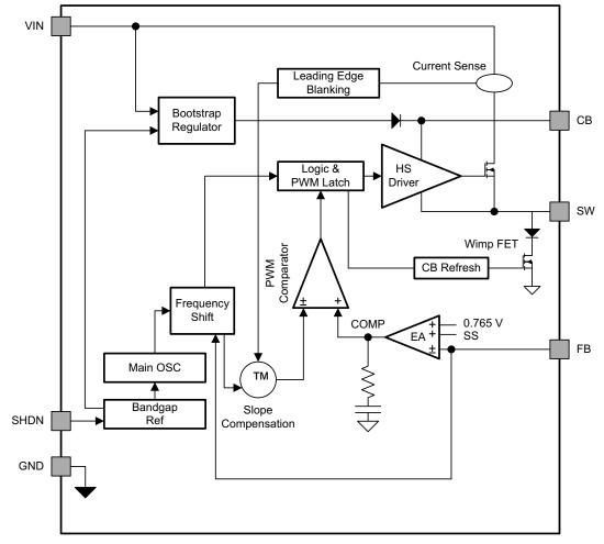
Figure 5. LMR16006 Functional Block Diagram
