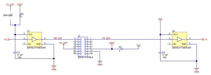
Figure 13. UART Interface Connector Schematic
