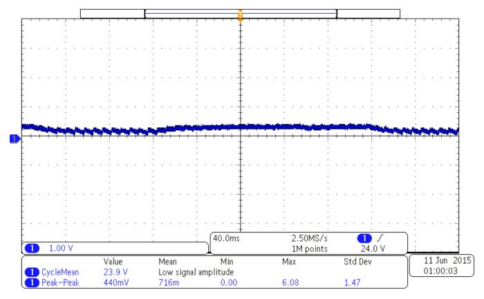
Figure 24. Ripple Voltage at C15 for an 18-V AC, 60-Hz Input
