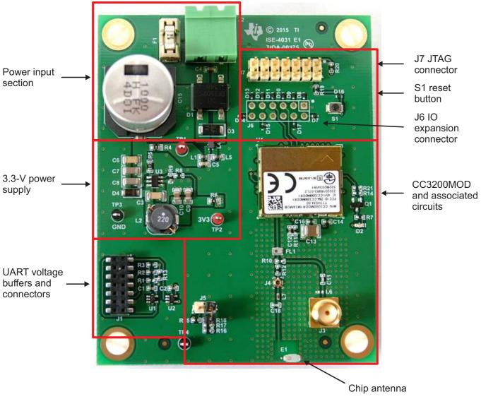
Figure 8. UART to Wi-Fi Bridge Printed Circuit Board Partition
