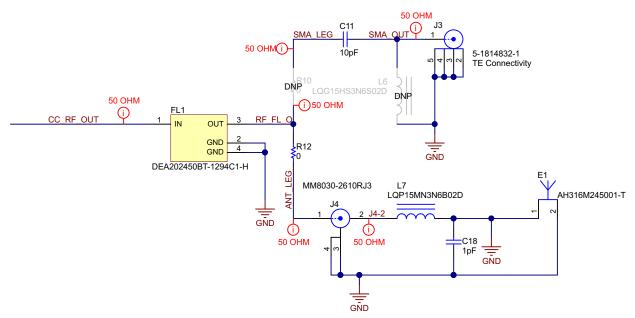
Figure 12. Antenna Section Schematic
