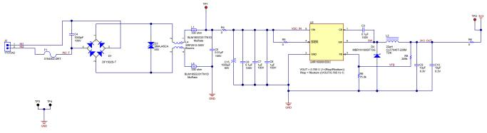
Figure 9. Power Input and 3.3-V Power Supply Schematic
