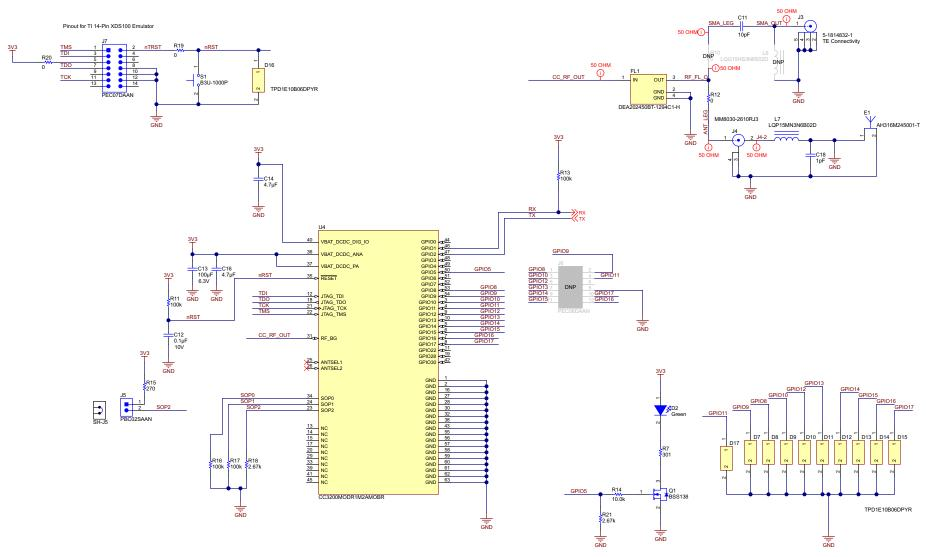
Figure 30. CC3200MOD Schematic
