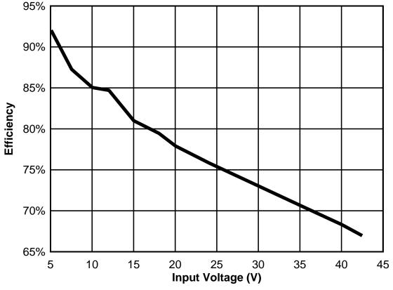
Figure 22. Power Supply Efficiency for UART Sending Data Continuously
