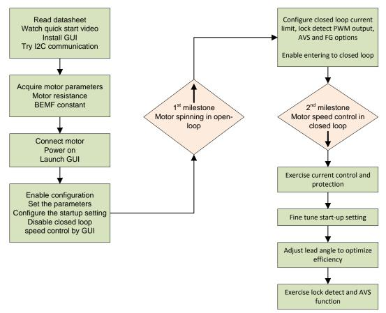
Figure 13. Events for Tuning Motor Parameters for DRV10983
