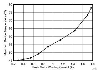
Figure 41. Peak Winding Current versus Maximum Temperature Observed on DRV10983
