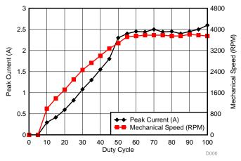
Figure 37. Duty Cycle Control versus Motor Speed
