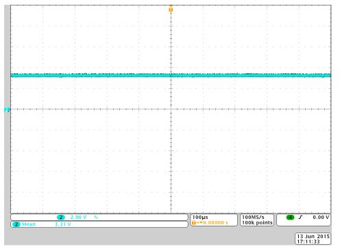
Figure 20. Voltage at DVDD Pin of DRV8303
