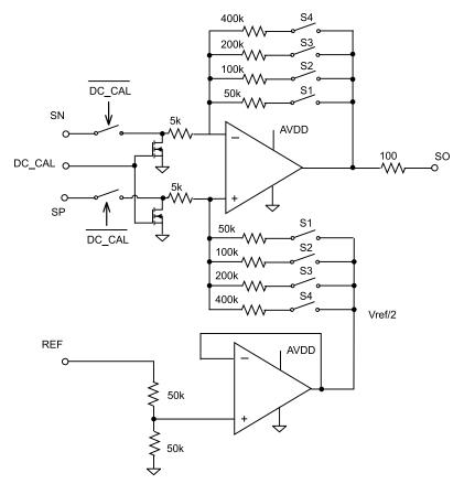
Figure 6. Current Shunt Amplifier in DRV8303 - Simplified Block Diagram
