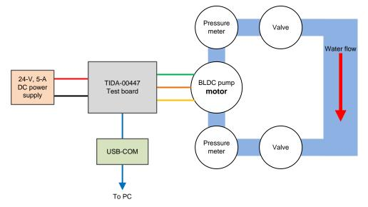
Figure 31. Block Diagram of Load Test Setup (Illustrated)
