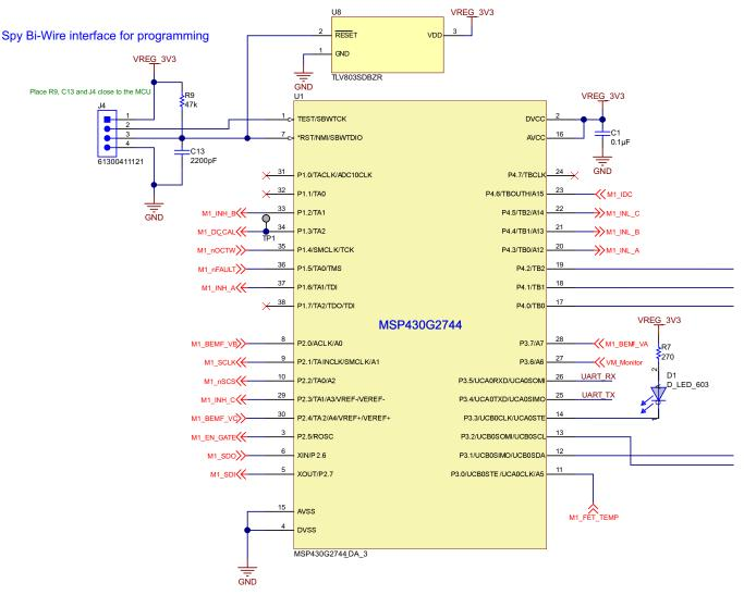
Figure 12. Pin Mapping for PWM Outputs on MSP430G2744
