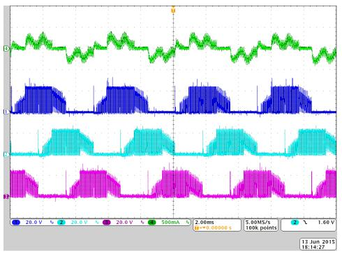
Figure 26. 3-Phase BEMF Voltage With Single Winding Current at PWM Duty of 50%
