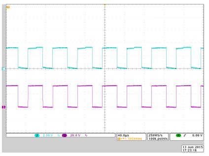
Figure 24. High-Side PWM Input and Output of DRV8303
