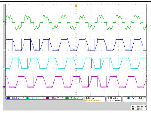
Figure 27. 3-Phase BEMF Voltage With Single Winding Current at PWM Duty of 100%
