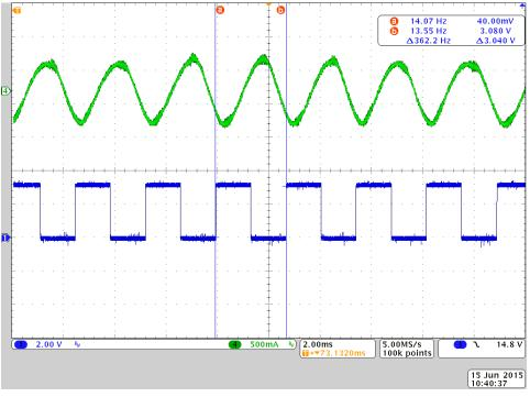
Figure 29. DRV10983 Speed Signal versus FG When FGcycle == 0x00
