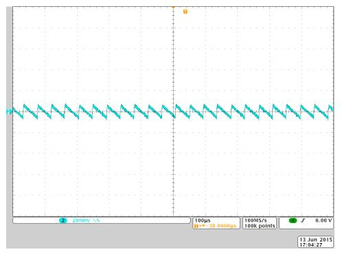
Figure 17. Ripple in 3.3-V Output From the Step-Down Regulator of DRV10983
