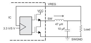
Figure 11. DRV10983 Step-Down Voltage Regulator
