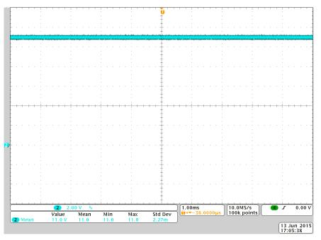
Figure 18. Voltage at GVDD Pin of DRV8303
