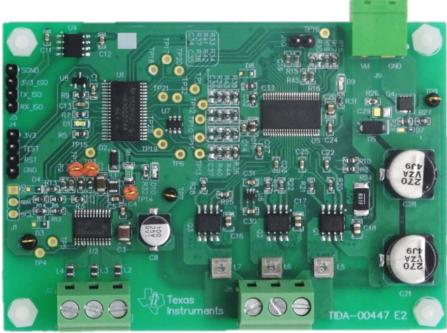
Figure 14. Assembled Control Unit—Top View
