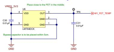
FET temperature sensing circuit
