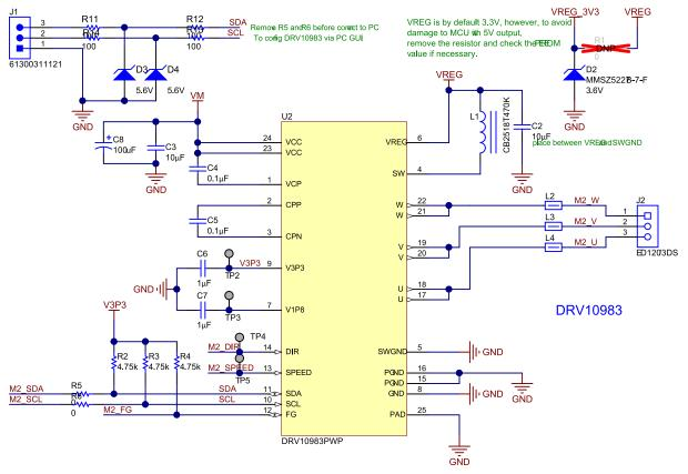
Figure 10. DRV10983 Circuit Schematic
