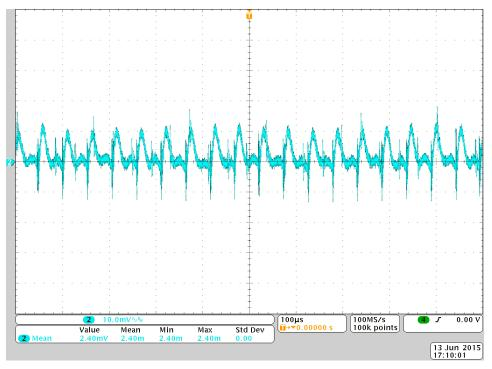
Figure 21. Ripple at DVDD Pin Voltage of DRV8303
