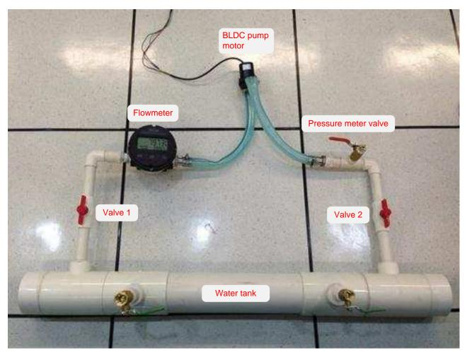
Figure 32. Block Diagram of Load Test Setup (Photo)
