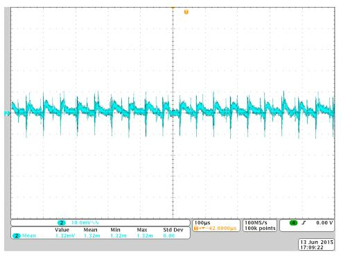
Figure 23. Ripple at AVDD Pin Voltage of DRV8303
