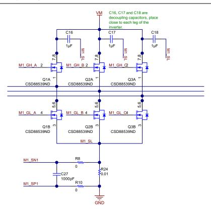
Figure 4. Three-Phase Inverter of Power Stage
