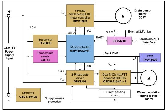
Figure 2. Block Diagram of Driver Unit
