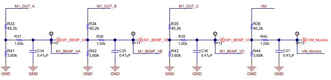
Figure 7. Motor Winding Voltage Sense Circuit
