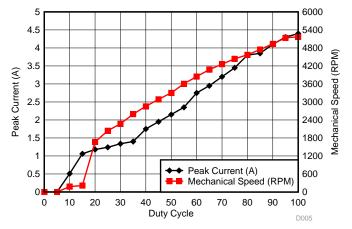
Figure 35. Speed Signal Duty versus Motor Speed
