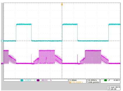
Figure 25. High-Side Gate-to-Ground versus Low-Side Gate-to-Source Signal From the DRV8303
