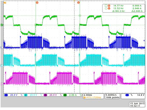
Figure 36. Phase Current Against 3-Phase Voltage With Load on DRV8303
