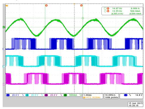
Channel 1: FG signal from DRV10983; Channel 3: Winding current.
