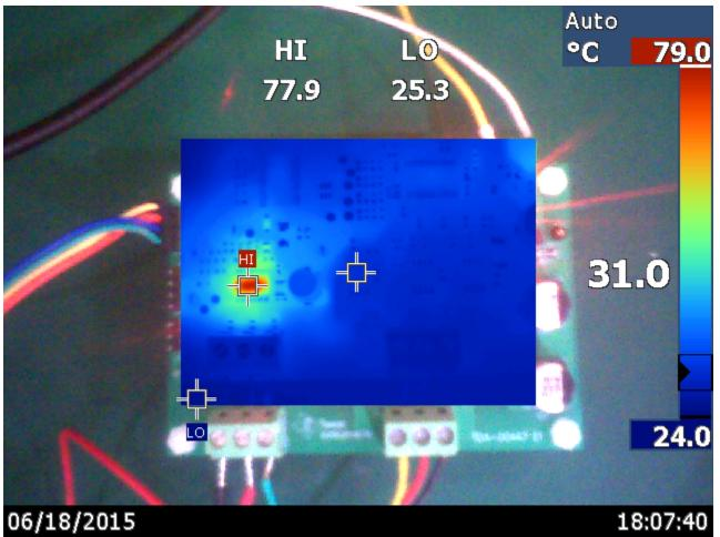
Figure 39. Load Test at 24 V—Thermal Image of Board at Winding Current of 1.77 APEAK
