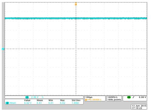
Figure 22. Voltage at AVDD Pin of DRV8303
