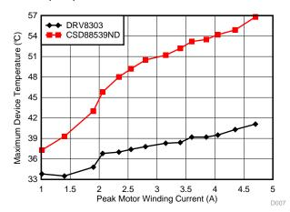
Figure 40. Peak Winding Current versus Maximum Temperature Observed on DRV8303 and CSD88539ND
