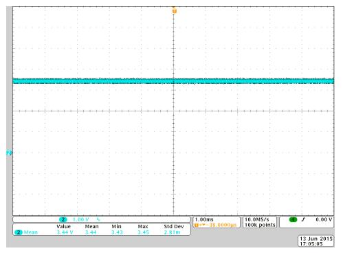
Figure 16. Output Voltage of 3.3 V From the Step-Down Regulator of DRV10983
