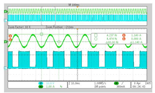
Figure 34. Load Test of DRV10983—Winding Current and Winding Voltage Measured With Respect to Negative DC Bus
