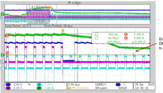
Due to latch protection, DRV8303 stops output to the gate FETs
