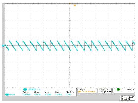
Figure 19. Ripple at GVDD Pin Voltage of DRV8303
