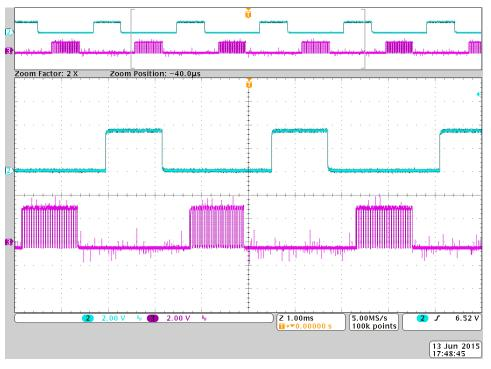
Figure 28. MCU Output Signals to DRV8303 on the Same Leg of Inverter Circuit
