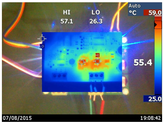
Figure 38. Load Test at 24 V—Thermal Image of Board at Winding Current of 4.7 APEAK
