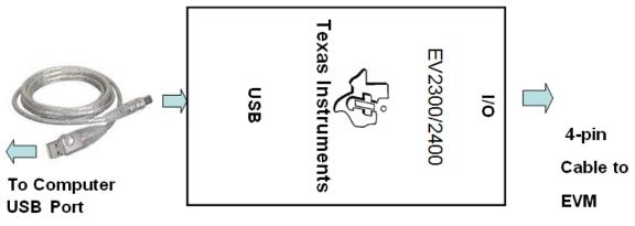
Figure 1. Connections of the EV2300/2400
