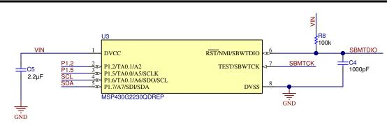
Figure 4 Schematic of the MCU
