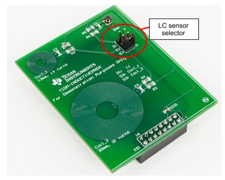
Figure 12. LC Sensor Selector
