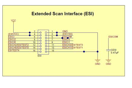
Figure 27. LC Sensor Board Schematic
