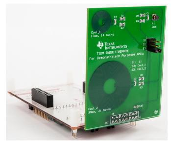
Figure 10. Sensor Board and LaunchPad Connection (Rev. 1.0)
