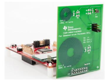
Figure 11. Sensor Board and LaunchPad Connection (Future Revisions After Rev. 1.0)
