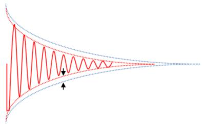
Figure 8. Maximum Difference Along the Decaying LC Signal
