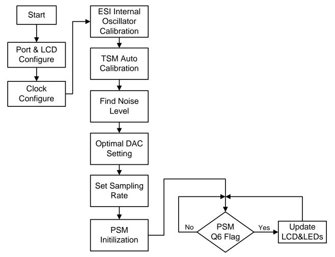
Figure 15. Flow Chart of the Software
