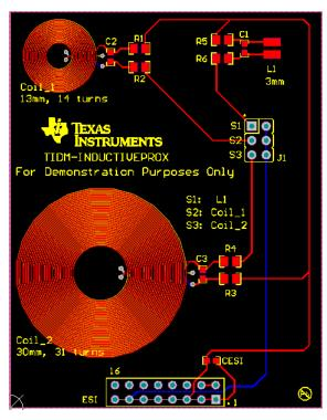
Figure 34. LC Sensor Board Layout
