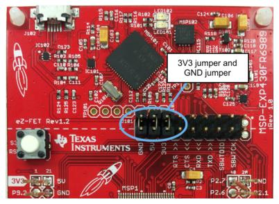
Figure 20. USB Power Supply Jumper Configuration
