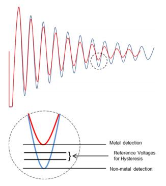
Figure 9. Reference Voltages for Detection of LC Signal to Identify Metal and Nonmetal Parts
