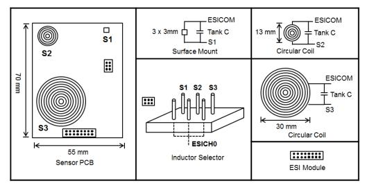
Figure 3. LC Sensor Board Diagram
