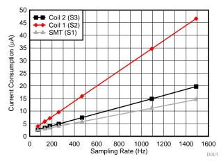
Figure 23. System Power Consumption With LPM2
