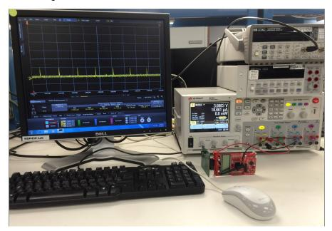
Figure 22. Power Consumption Test Configuration
