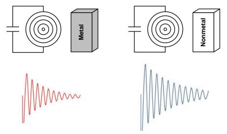
Figure 7. LC Oscillation Signal of Detection for Metal and Nonmetal
