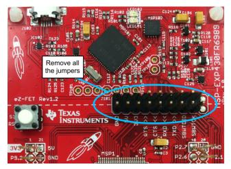
Figure 17. External Power Supply Jumper Configuration
