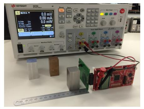
Figure 18. DC Power Analyzer Distance Test Configuration
