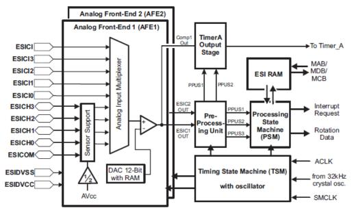
Figure 4. Block Diagram of the ESI
