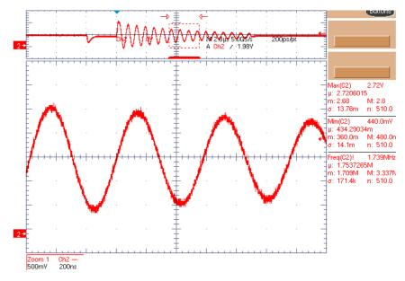
Figure 26. SMD Oscillation Waveform
