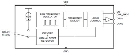
Figure 4: TPL5111 Functional Block Diagram
