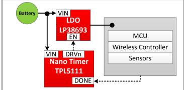
Figure 2 TIDA-00720 High Level Block Diagram
