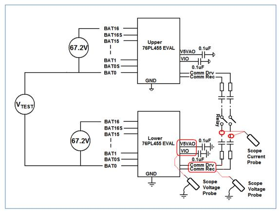
Figure 12. Communication Cable Insertion Hot-Plug Test Setup
