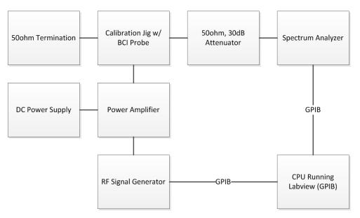
Figure 2. Calibration Block Diagram
