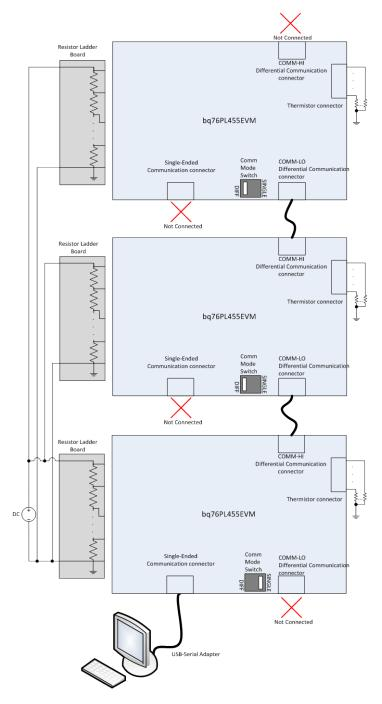
Figure 1. Test Setup
