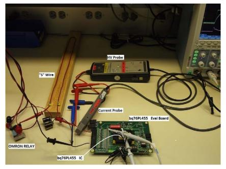
Figure 7. Single Board Hot-Plug Test Setup
