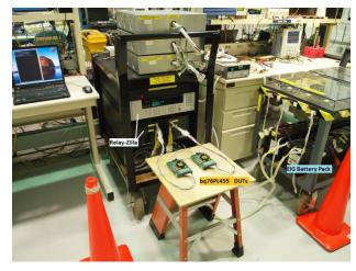
Figure 8. Stacked Boards Hot-Plug Test Setup
