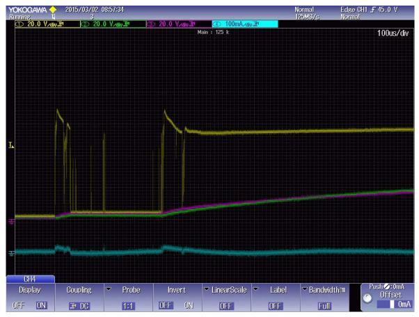
Figure 10. Scope Capture (VTEST = 80 V Across BAT16 → BAT0)
