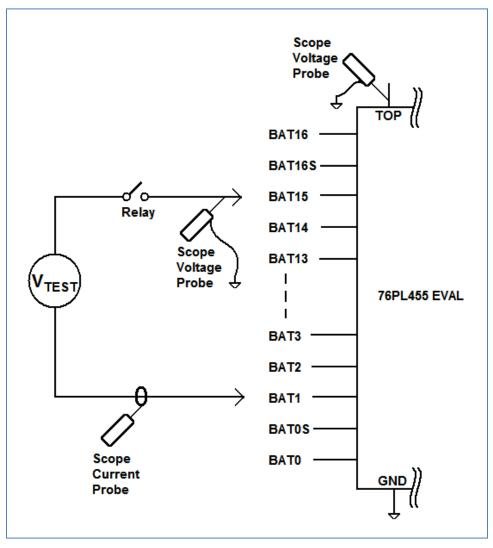
Figure 9. Single Board Power Cable Insertion Hot-Plug Test Setup
