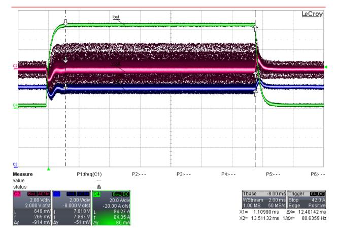
Transient at 8Vin, 0A-to-84A load step at ≈ 0.5A/μsec
