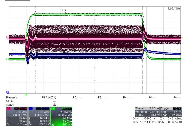
Transient at 7Vin, 0A-to-84A load step at ≈ 0.5A/μsec
