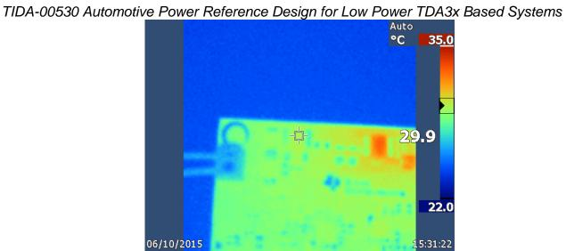
Figure 32: LM74610 (reverse polarity protection) FET, no load
