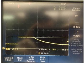
Figure 51: Pulse 5b (clamped load dump) test pulse
