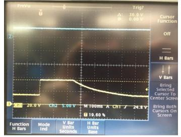
Figure 52: WVIN output is undisturbed during load dump pulse
