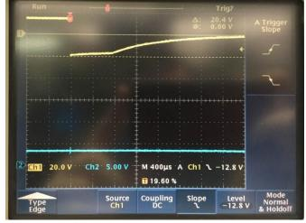
Figure 45: TVS circuit clamps the negative voltage to -20.4V
