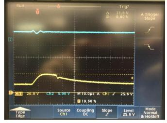
Figure 49: TVS circuit clamps voltage to 31.6V
