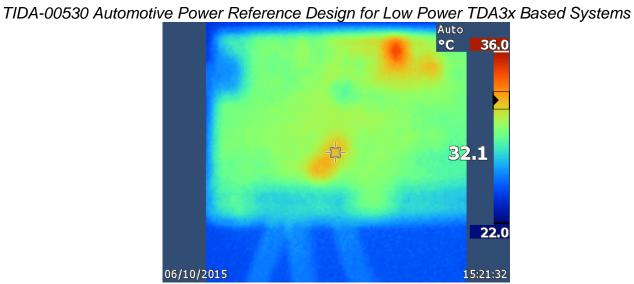
Figure 40: VDDQ IC, full load, steady state
