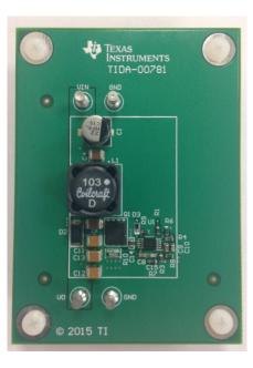
Figure 1 Reference board top view
