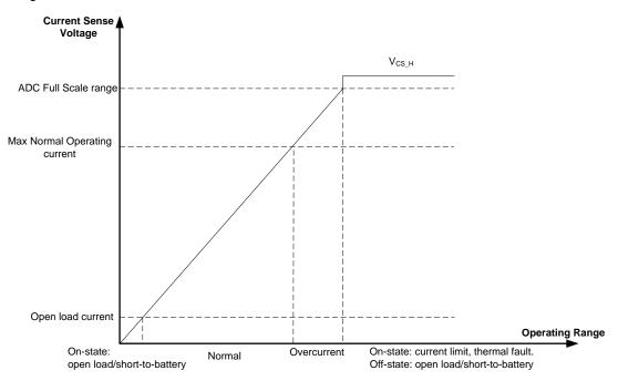
The following Figure 3 shows a typical current sense voltage according to the operating conditions, including fault conditions.
