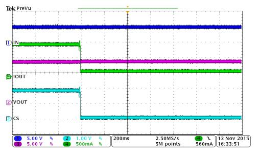
Figure 8. Output Open Load or Short-to-Battery
