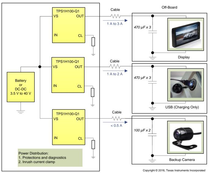
Figure 1. System Block Diagram of Inrush Current Clamping
