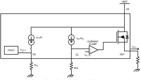
Figure 2. Current Sense and Current Limit Functions
