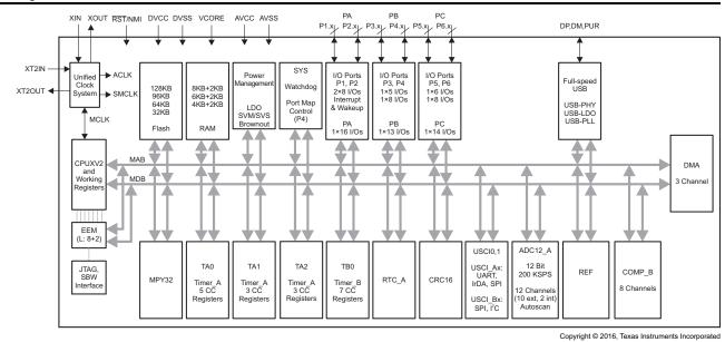
Figure 4. MSP430F5528 Functional Block Diagram
