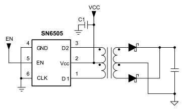
Figure 9. Unregulated Isolated DC/DC Converter Using SN6505
