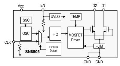
Figure 3. SN6505 Functional Block Diagram
