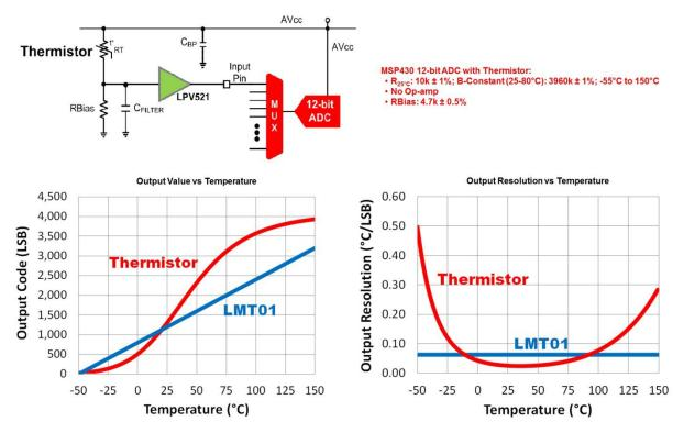
Figure 10. Output Code and Output Resolution versus Temperature
