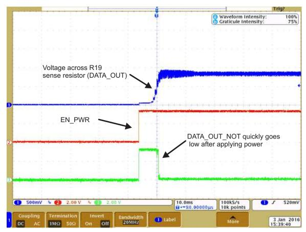
Figure 27. Circuit Behavior During Short Circuit Fault Between Sensor Leads
