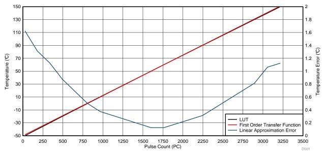
Figure 21. LMT01 Output Transfer Function and Accuracy With Linear Approximation
