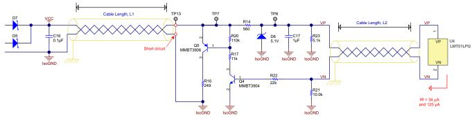
Figure 28. Short Circuit in 8-V Rail Wires
