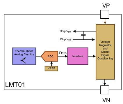
Figure 2. LMT01 Functional Block Diagram
