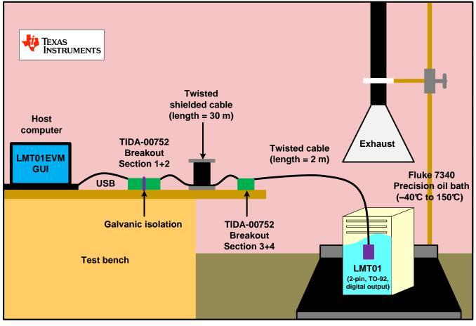
Figure 36. Oil Bath Test Setup
