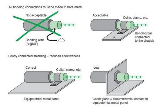
Figure 41. Implementations of Shielded Cables
