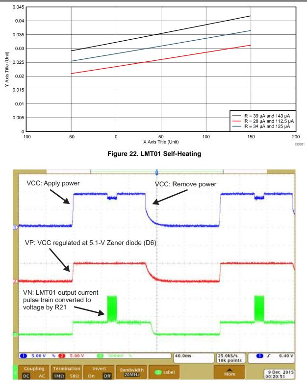
Figure 23. VCC (Trace-1), VP (Trace-2), and VN (Trace-3) Waveforms
