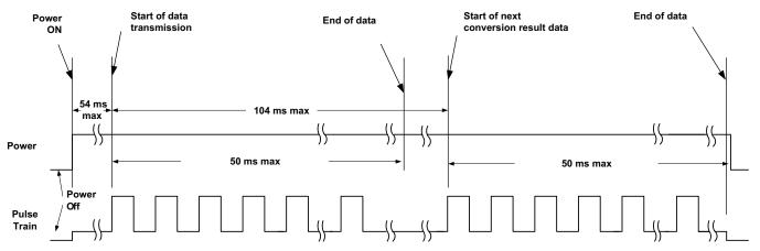
Figure 16. Temperature to Digital Pulse Train Timing Cycle
