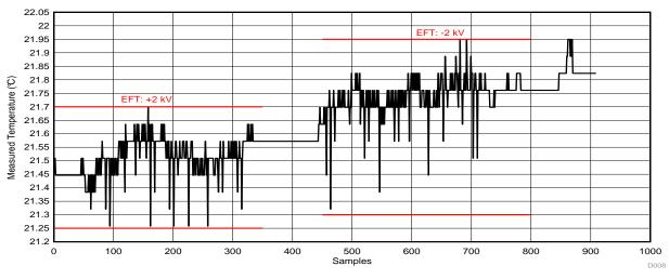
Figure 40. Performance During EFT Immunity Test Using Shielded Twisted Pair Cable
