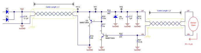
Figure 25. Open Circuit Connection on Sensor Leads
