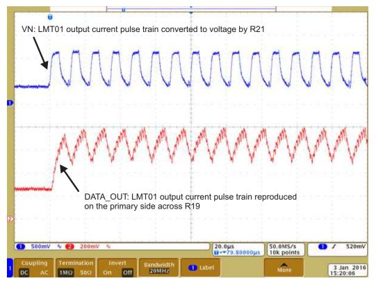
Figure 19. VN (Trace-1) and DATA\_OUT (Trace-2) Waveforms
