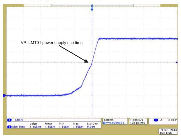
Figure 34. LMT01 Power Supply Rise Time
