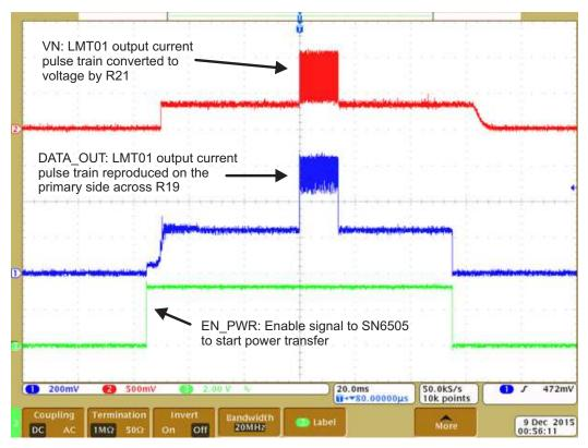
Figure 18. VN (Trace-2), DATA\_OUT (Trace-1), and EN\_PWR (Trace-3) Waveforms
