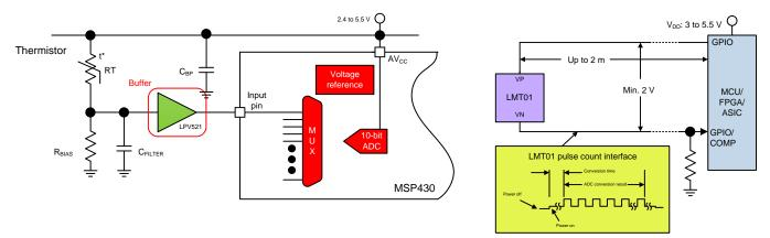
Figure 12. Typical Thermistor and LMT01-Based Circuits
