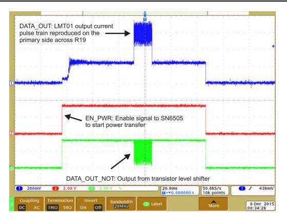
Figure 20. DATA\_OUT (Trace-1), EN\_PWR (Trace-2), and DATA\_OUT\_NOT (Trace-3) Waveforms
