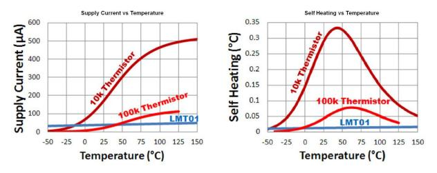
Figure 11. Supply Current and Self Heating versus Temperature
