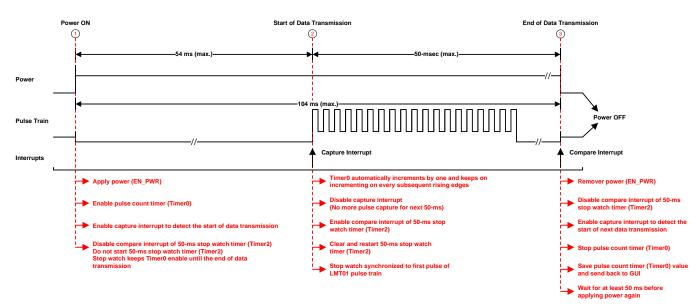
Figure 33. Flow Diagram for Two Timers Synchronous Transistor Mode Pulse Counting Method
