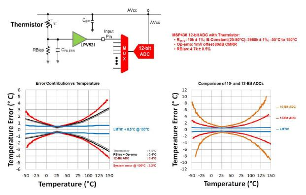
Figure 13. Thermistor and LMT01 Error Contribution versus Temperature
