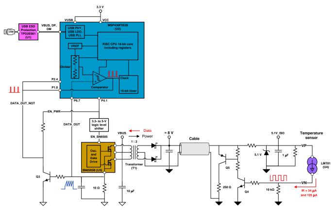
Figure 1. Conceptual Schematic Diagram of 2-Wire Galvanically Isolated IC Temperature Sensor With Pulse Count Interface (TIDA-00752)
