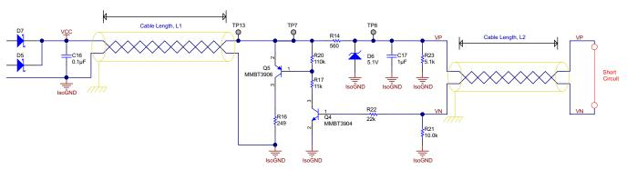
Figure 26. Short Circuit Between Sensor Leads
