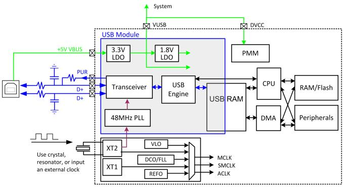
Figure 8. Powering MSP430 From USB Using Internal LDO
