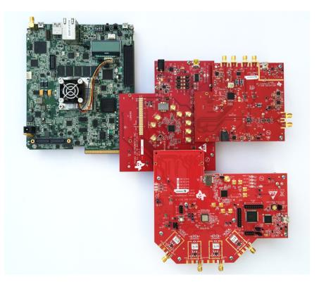
Figure 5. 66AK2L06 DSP+ARM Processor JESD204B Attach to ADC14X250 / DAC38J84 Design Development Kit
