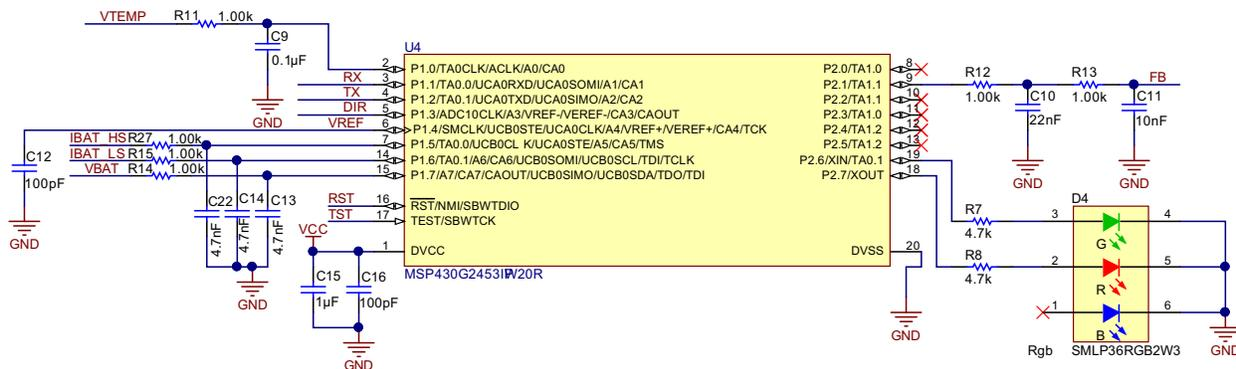
Figure 6. Microcontroller Section
