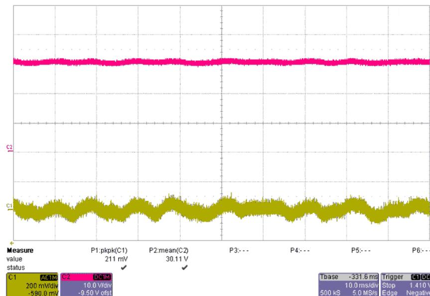
Figure 35. Output Voltage and Current (AC Coupled) in CC Region
