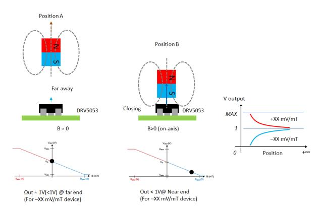
The magnet and Hall sensor configuration to get non-linear response to the position
