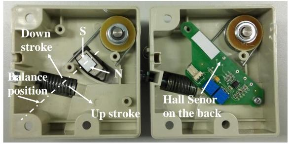
Figure 4. Foot pedal structure
