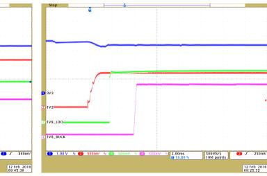
Figure 80. Startup Behavior of 1V2, 1V8\_LDO, and 1V8\_BUCK When Activated By Ignition Switch With 3V3 Main Rail Already Powered On
