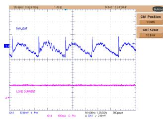
Figure 53. TPS61170-Q1 5.0-V Rail Ripple Voltage With 100-mA Load
