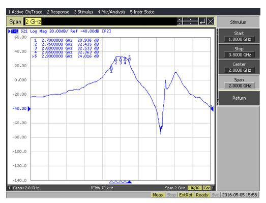
Figure 12. RF Front-End Gain Measurement (S21)
