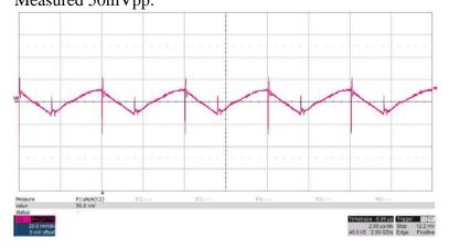
5V Ripple (C12) 20mV/div, 2usec/div Measured 42mVpp:
