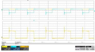
Q5 drain to source with 57V input, 1A load, and 200MHz BWL Measured 18.3Vpeak:
