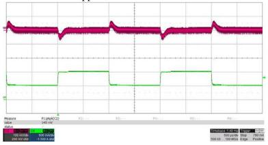
3.3V load step, 5V response Measured 163mVpp across C12:
