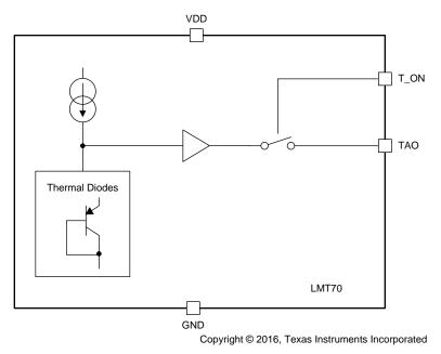
Figure 2. LMT70 Block Diagram
