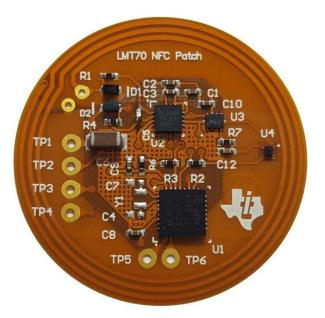
Figure 6. NFC Temperature Patch Reference Design
