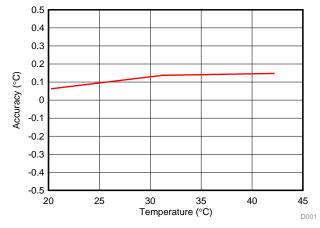
Figure 11. NFC Temperature Sensor Patch Accuracy at Human Body Temperatures
