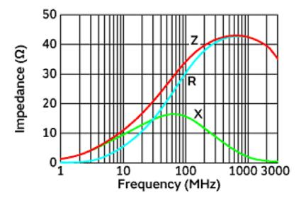
Figure 3. Impedance VS. Frequency Characteristics (BLM21PG300SN1)
