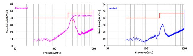
Figure 5. Radiated EMI Result (V<sub>IN</sub>=3.3V, V<sub>0</sub>=5V/I<sub>0</sub>=3A)
