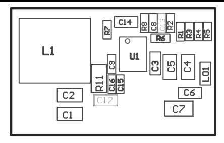
Figure 13. PMP9778 Assembly Drawing
