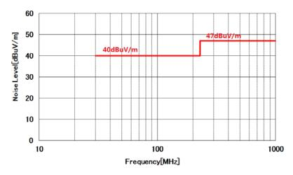
Figure 1. EN55022 and CISPR22 Class B Radiated Emission Limit
