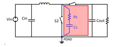
Figure 2. Critical Current Path of Boost Converter
