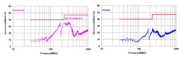
Figure 7. Radiated EMI Result (V<sub>IN</sub>=3.3V, V<sub>0</sub>=12V/I<sub>0</sub>=1.5A)
