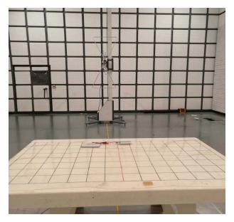
Figure 4. Setup of the Radiated EMI Test
