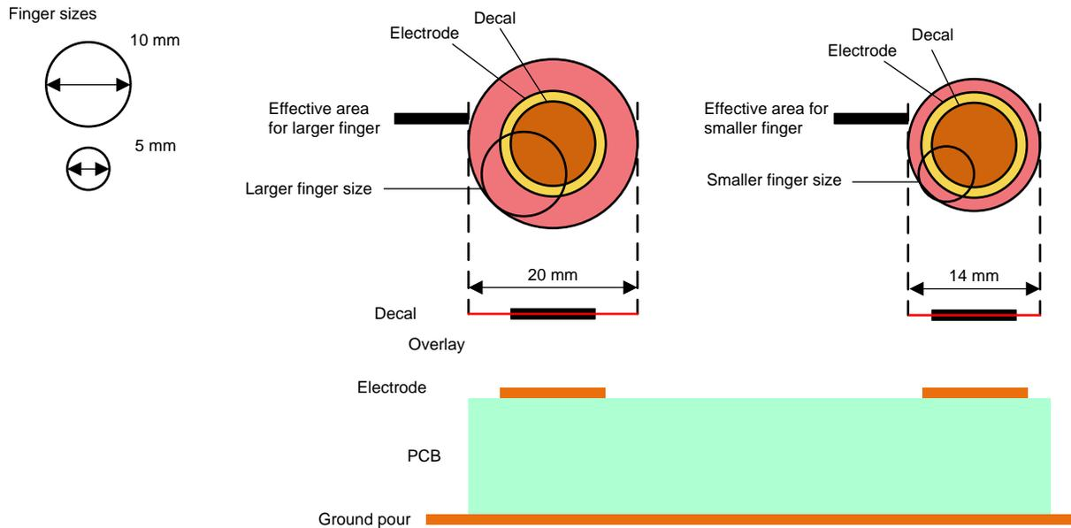
Figure 9. Effective Area Example for Electrodes Larger Than Decal
