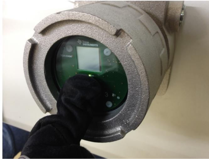
**Figure 21. Touch With Gloves Test**
