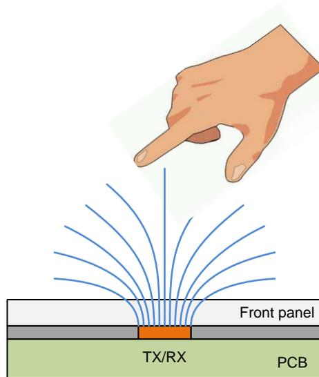
**Figure 7. Self Capacitive Button Designs Example**
