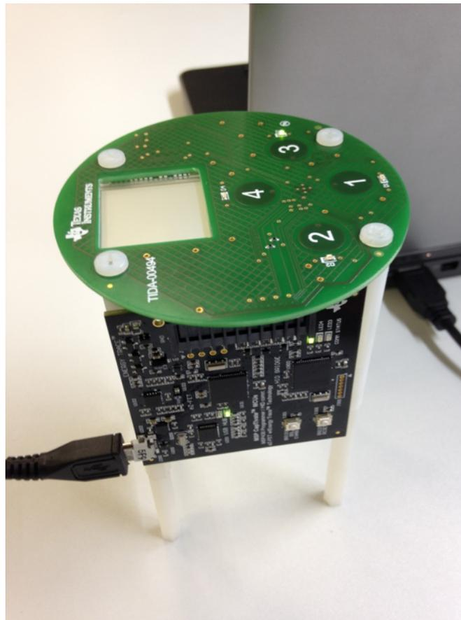
**Figure 14. TIDA-00494 Connected to the PC, Ready for Data Acquisition and Debugging**
