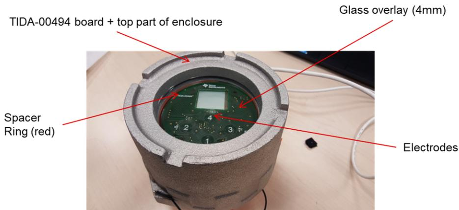
**Figure 26. Test Setup**
