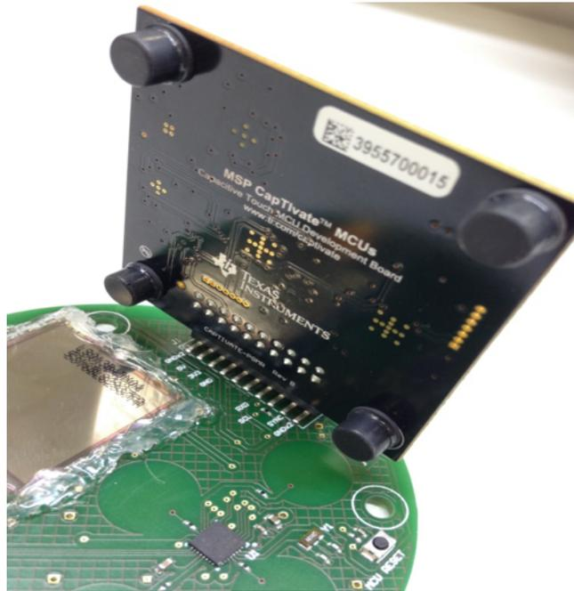
**Figure 13. TIDA-00494 Connected to the CAPTIVATE-PGMR PCB**
