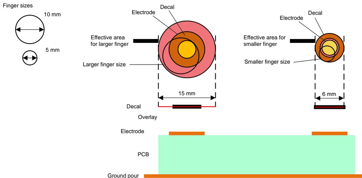
Figure 10. Effective Area Example for Electrode Smaller Than Decal
