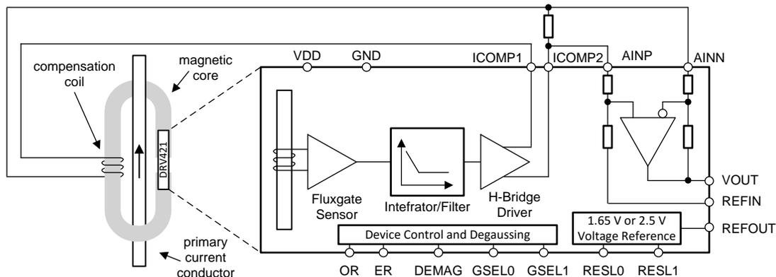
Figure 4. Closed Loop System Using DRV421 With Integrated Fluxgate Sensor
