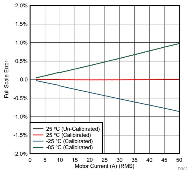
Figure 13. Full Scale Error versus Motor Current
