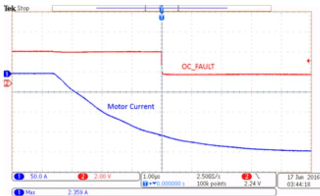
Figure 24. Overcurrent Detection for Negative Current
