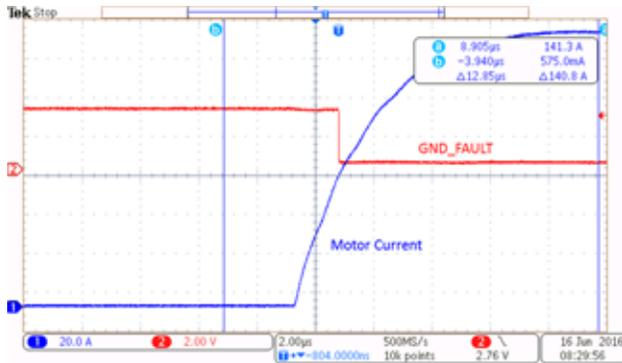
Figure 26. Ground Fault Detection for Positive Current
