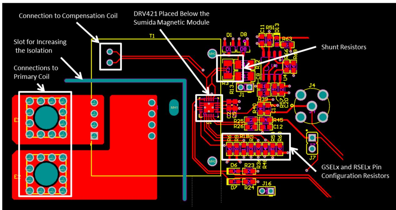
Figure 30. Layout Selection for Sumida Module and DRV421
