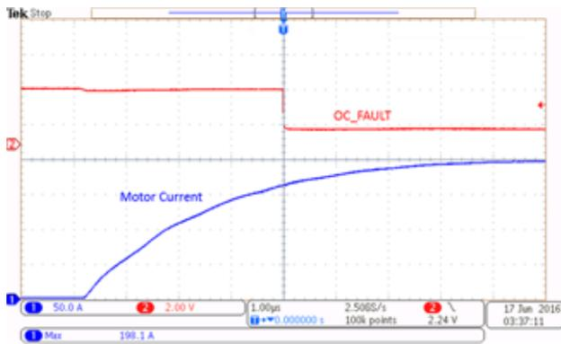
Figure 22. Overcurrent Detection for Positive Current
