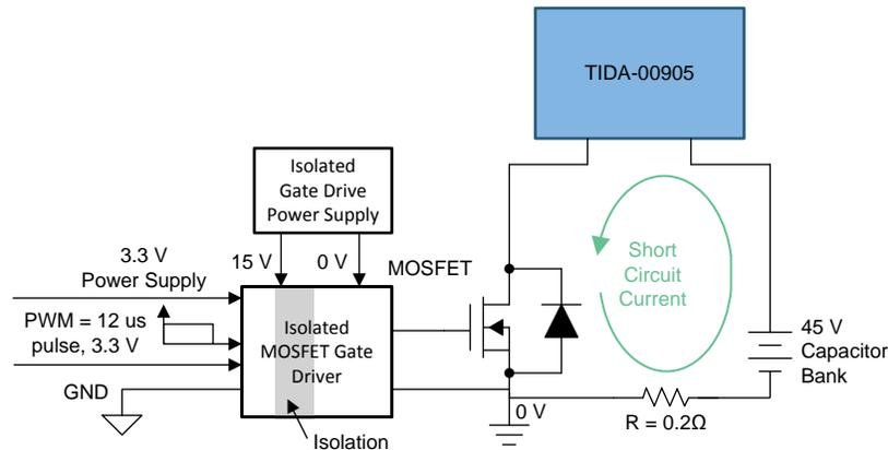
**Figure 21. Short-Circuit Test Diagram**
