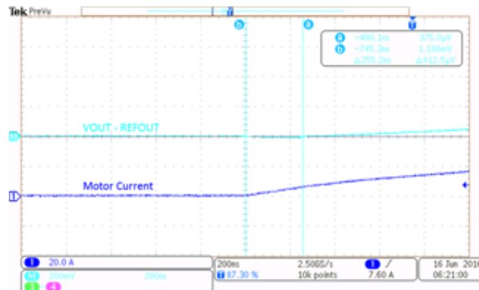
Figure 20. Step Response and Propagation Delay Time
