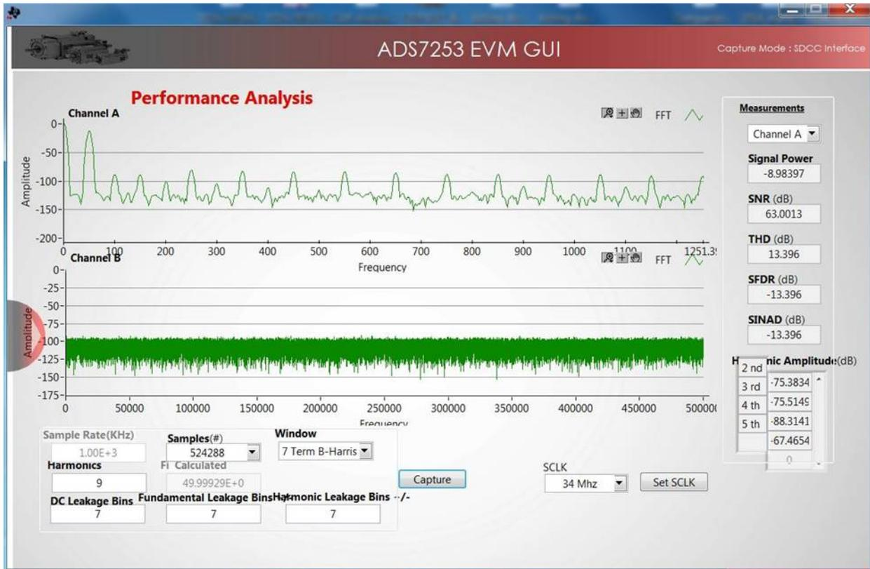
Figure 18. Spectrum of Captured Data Noise and Fundamental
