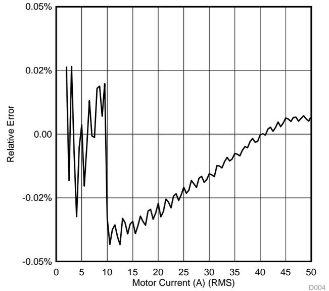
Figure 15. Relative Error versus Motor Current Calibrated at 25°C
