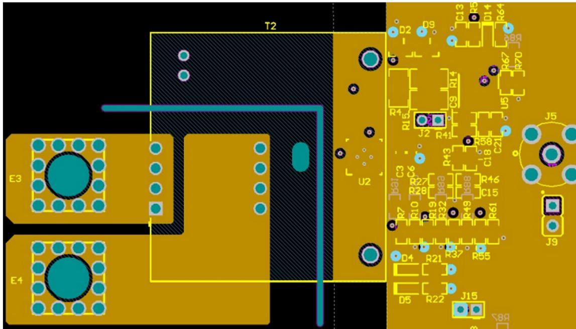
Figure 31. Power Layer for TIDA-00905
