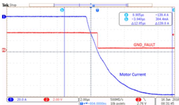
Figure 28. Ground Fault Detection for Negative Current
