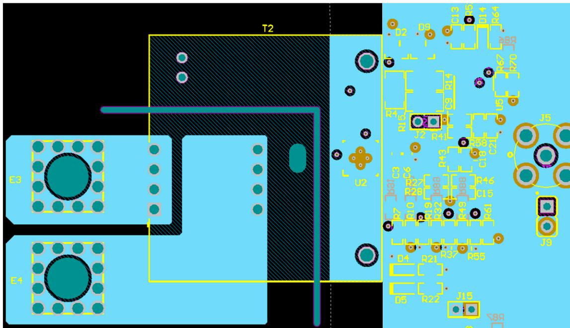
Figure 32. GND Layer for TIDA-00905
