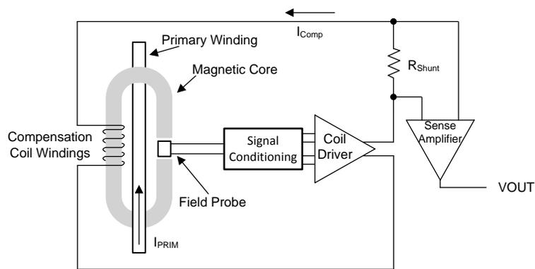
**Figure 3. Closed-Loop Sensor Block Diagram**
