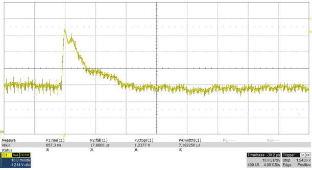
Waveform across 10 mOhm dynamic load tied to ground: 260mV decrease in less than 500nsec Close in tip & barrel at added 10mOhm tied to ground and source of CSD16322 (drain of CSD16322 to Vout, gate has 1k to ground and is driven by Tektronix AFG3102 generator, with pulse of 1 msec wide every 20 msec, pulse high 1.265V x2, pulse low 0V, "leading" and "trailing" each 1.00 usec) 20 MHz BW
