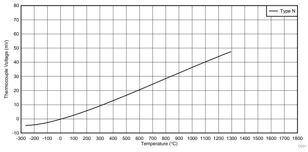
Figure 3. Thermocouple Voltage as Function of Temperature
