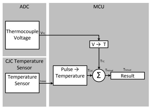
Figure 14. Software Flow Diagram
