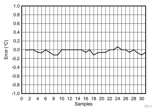
Figure 26. LMT01-Q1 Temperature Error at 0°C
