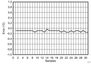
Figure 25. LMT01-Q1 Temperature Error at -35°C
