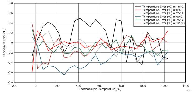
Figure 24. Thermocouple Channel Plus CJC Error in °C With Gain and Offset Calibration
