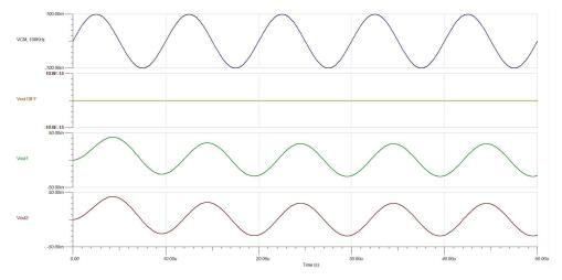
Figure 7. Differential Noise Due to Mismatches in Common-Mode Capacitors
