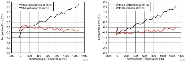
Figure 17. Temperature Error at 25°C for TC Channel
