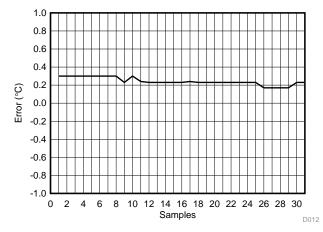
Figure 27. LMT01-Q1 Temperature Error at 25°C
