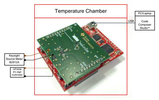
Figure 15. Testing Equipment Connection
