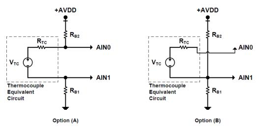
Figure 8. Thermocouple Biasing Options Using Pullup and Pulldown Resistors
