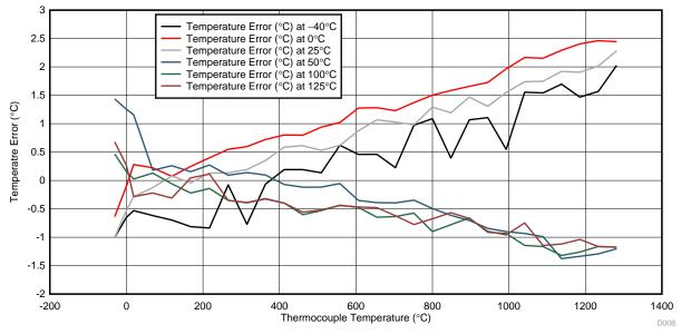
Figure 23. Thermocouple Channel Error in <sup>o</sup>C Without Gain and Offset Calibration
