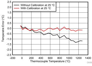
Figure 21. Temperature Error at 75°C for TC Channel
