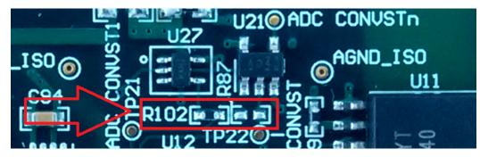
Figure 24. Resistor Jumper
