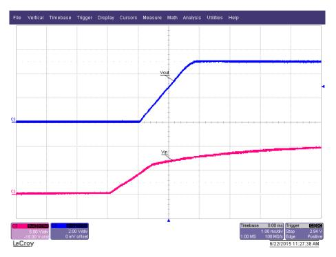
The photo below shows the output voltage startup waveform after the application of 10.8V in with the 5V output loaded to 2A. (Vout: 5V/DIV, 1mS/DIV), (Vin: 2V/DIV)
