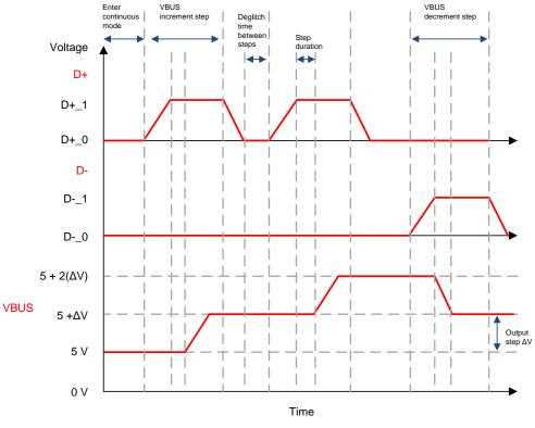
Figure 8. Adjustable Adapter-Output Steps
