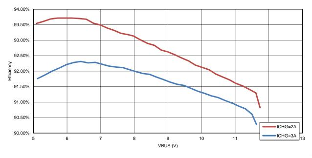
Figure 9. BQ25890H Charge Efficiency Using Anker QC3.0 Adapter
