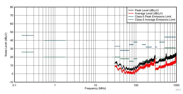
Figure 20. Radiated Emissions of 30 MHz to 1000 MHz
