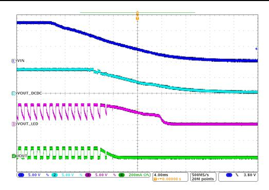
Figure 12. Shut Down:  $V_{IN} = 12 \text{ V}$ , Duty Cycle = 50%
