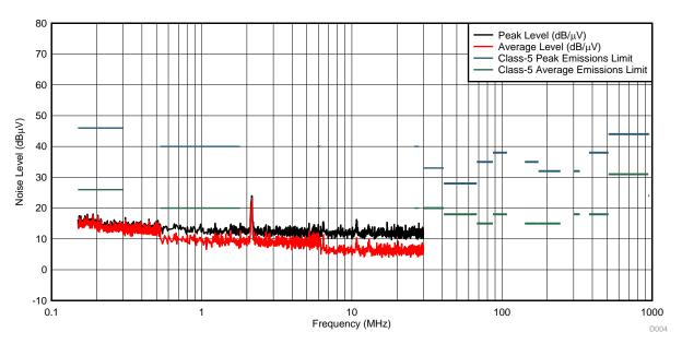
Figure 19. Radiated Emissions of 150 kHz to 30 MHz
