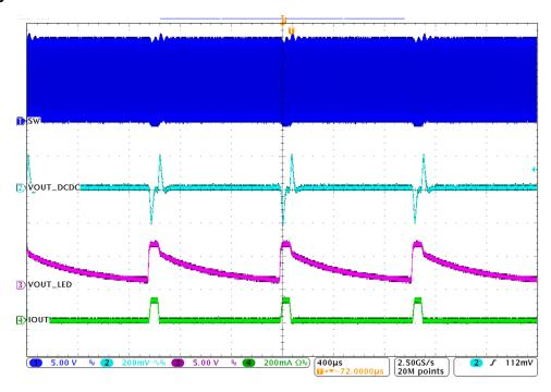
Figure 14. Steady State:  $V_{IN}$  = 12 V, Duty Cycle = 5%
