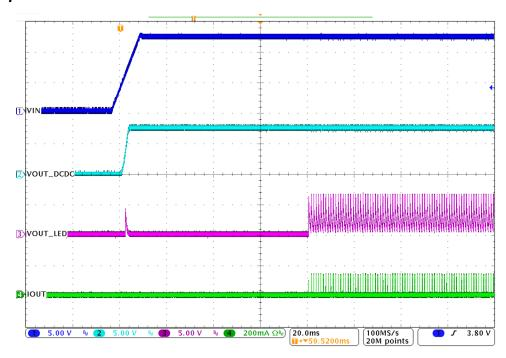
Figure 8. Start-Up:  $V_{IN} = 12 \text{ V}$ , Duty Cycle = 5%
