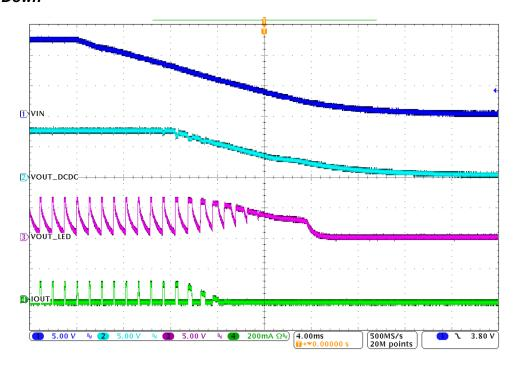
Figure 11. Shut Down:  $V_{IN} = 12 \text{ V}$ , Duty Cycle = 5%
