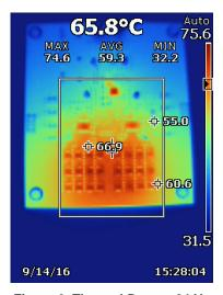
Figure 6. Thermal Data at 24 V<sub>IN</sub>
