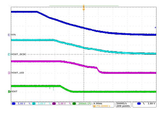
Figure 13. Shut Down:  $V_{IN}$  = 12 V, Duty Cycle = 100%
