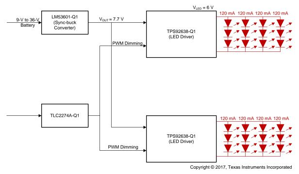
Figure 1. TIDA-01348 Block Diagram
