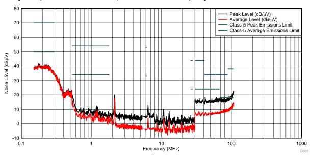
Figure 17. Conducted Emissions Positive
