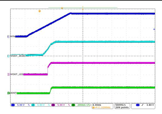
Figure 10. Start-Up:  $V_{IN}$ = 12 V, Duty Cycle = 100%
