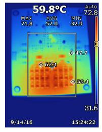
Figure 5. Thermal Data at 9 V<sub>IN</sub>
