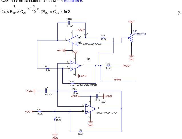
Figure 4. TLC2274A-Q1 PWM Generation Schematic
