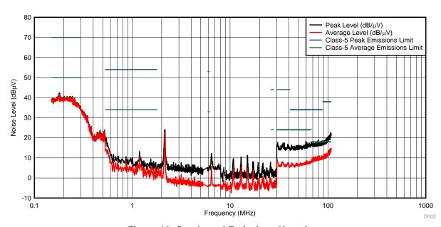
Figure 18. Conducted Emissions Negative
