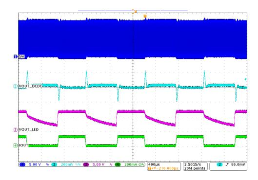
Figure 15. Steady State:  $V_{IN}$  = 12 V, Duty Cycle = 50%
