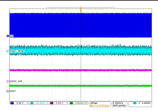
Figure 16. Steady State:  $V_{IN}$  = 12 V, Duty Cycle = 100%
