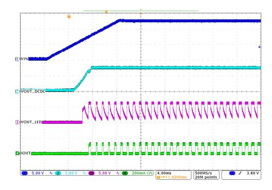
Figure 9. Start-Up:  $V_{IN} = 12 \text{ V}$ , Duty Cycle = 50%
