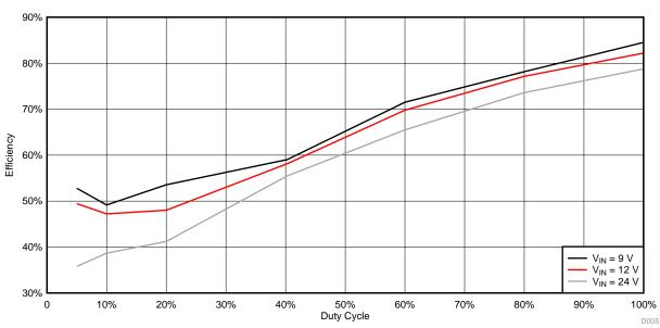
Figure 7. Efficiency versus Duty Cycle at Various Input Voltages
