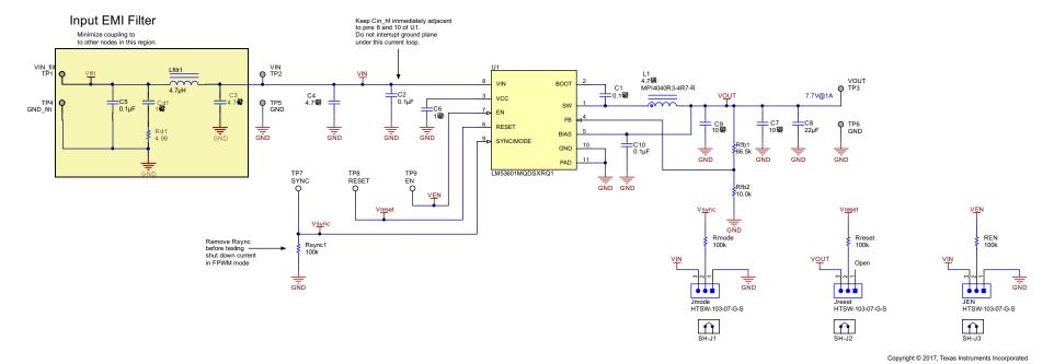
Figure 2. Buck Converter LM53601 Schematic
