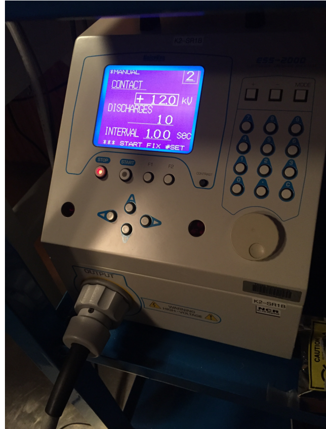
Figure 31. IEC61000-4-2 ESD Testing Configuration (12 KV With Interval of 1-s Voltage Spike Over 10-s Period)
