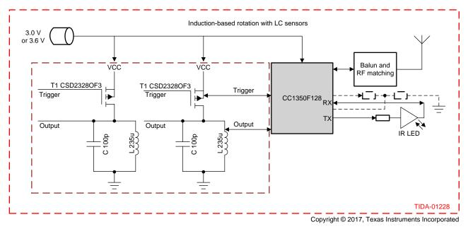
Figure 1. TIDA-01228 Block Diagram
