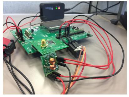
Figure 9. SRF06EB Wiring for EnergyTrace Measurements With FET430 Pro
