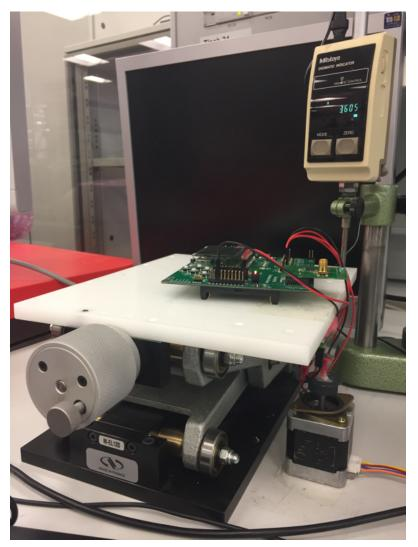
Figure 8. Stepper Motor With Disc at 3.6-mm Distance From TIDA-01228 (Face Down)
