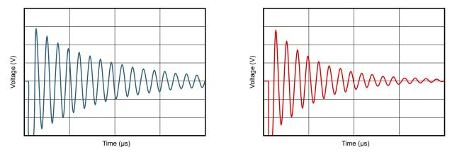
Figure 4. Dampened (to the right) and Undampened Oscillation of LC Sensor
