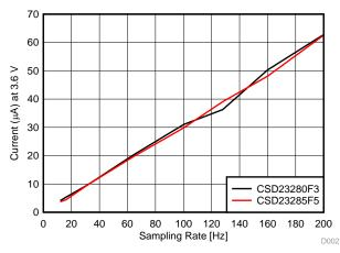
Figure 10. Power Consumption Comparison for Two FemtoFET Devices
