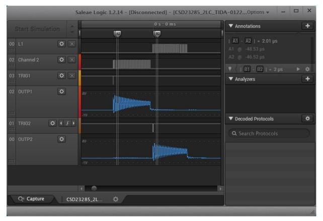
Figure 7. Undampened LCsensor1 and LCsensor2 Oscillation With Approximately 500 kHz Each
