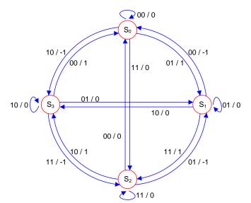
Figure 5. State Machine With 2-bit (LC Sensor 1 and LC Sensor 2) States S0 to S3
