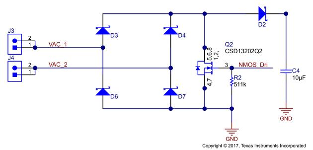
Figure 2. Rectifier and Overcharge Protection
