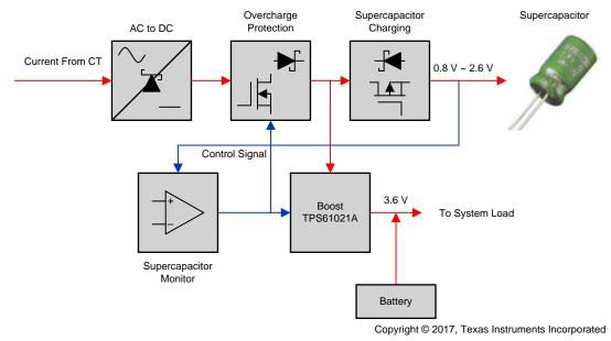
Energy Harvesting From Current Transformer With Supercapacitor for Fault Indicator Reference Design
