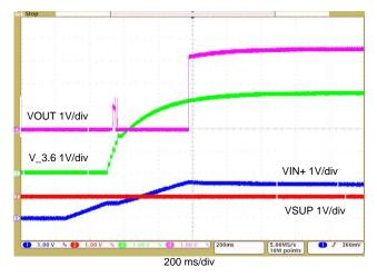
Figure 6. Startup With 3-mA Input Current and 4-k $\Omega$  Load
