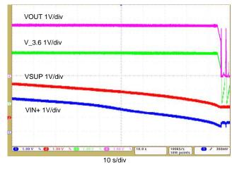
Figure 10. Supercapacitor Discharge Waveform With 50-mA Load
