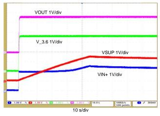
Figure 9. Supercapacitor Charging With 500-mA Input Current
