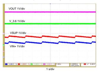
Figure 7. Overcharge Protection Measurement With 3-mA Input Current
