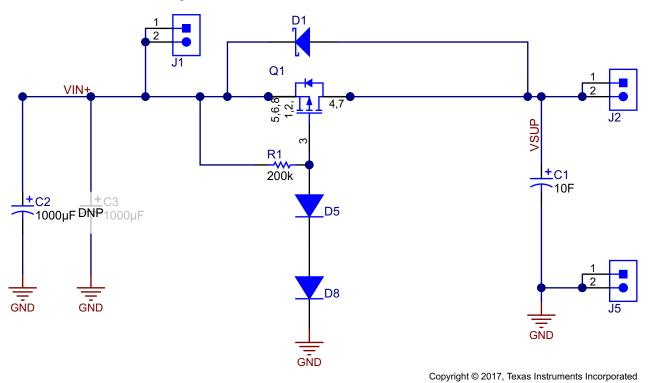
Figure 3. Schematic of Supercapacitor Charging Circuit
