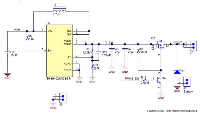
Figure 4. Schematic of Boost Converter Solution
