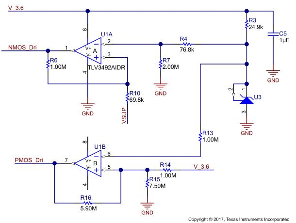
Figure 5. Schematic of Supercapacitor Protection Circuit
