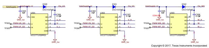
Figure 9. UCC27712-Q1 High- and Low-Side Gate Drivers
