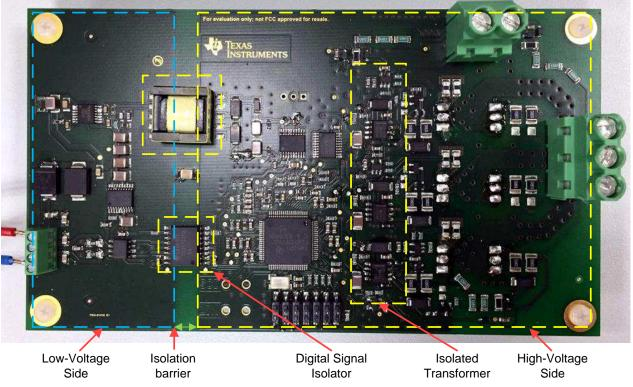
Figure 3. TIDA-01418 PCB—Top View (1)
