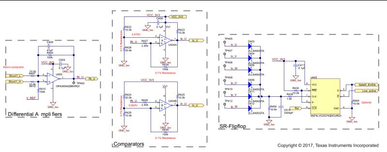
Figure 14. Overcurrent Protection Circuit
