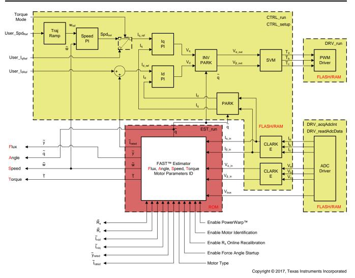
Figure 2. Block Diagram of InstaSPIN-FOC™
