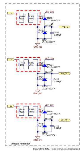
Figure 16. Motor Voltage Feedback Circuit
