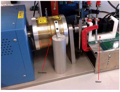
Figure 18. Three-Phase BLDC Motor and Dynamometer (Magtrol)
