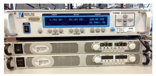
Figure 17. High-Voltage Power Supply (Agilent NS772A) and Power Analyzer (Magtrol 6530)
