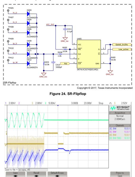
Figure 25. Overcurrent Condition
