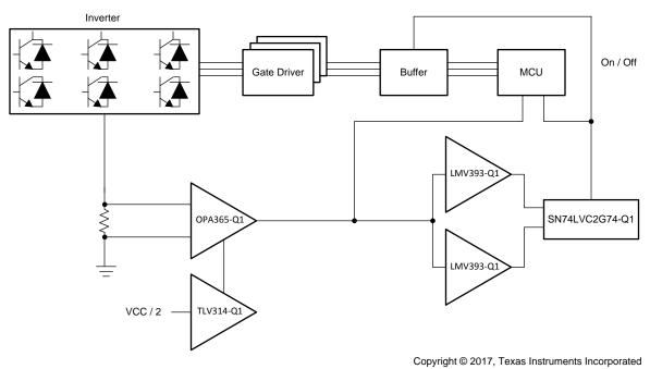
Figure 13. Block Diagram of Shunt Current-Monitoring Circuit
