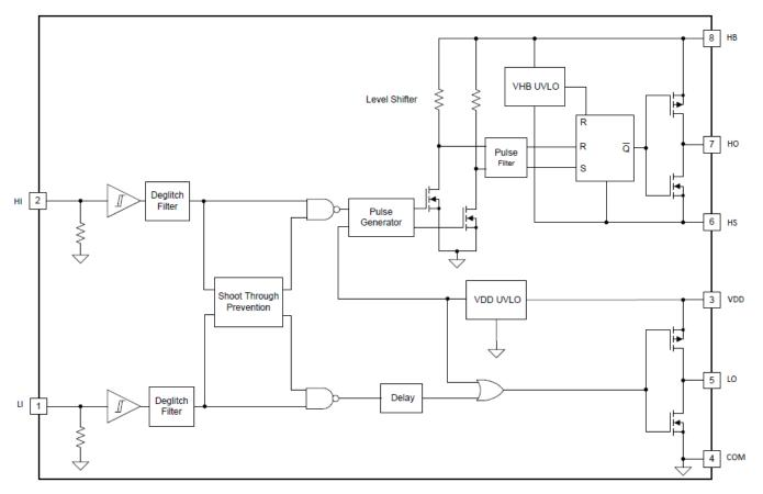
Figure 10. UCC27712-Q1 Functional Block Diagram
