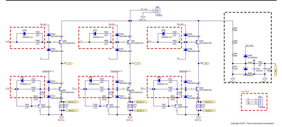
Figure 11. Three-Phase Inverter With Voltage Divider (Right Side) and Clamping Diodes to Measure Bus Voltage
